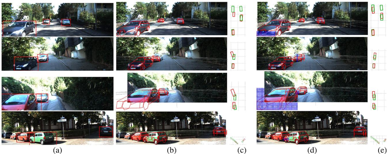
Fig. 9: FG+GP (a-c) vs FG+GP+DO+SO (d,e). (a) 2D bounding box detections, (b) FG+GP based on (a), (c) bird's eye view of (b), (d) FG+GP+DO+SO shape model fits (blue: estimated occlusion masks), (e) bird's eye view of (d). Estimates in red, ground truth in green.
