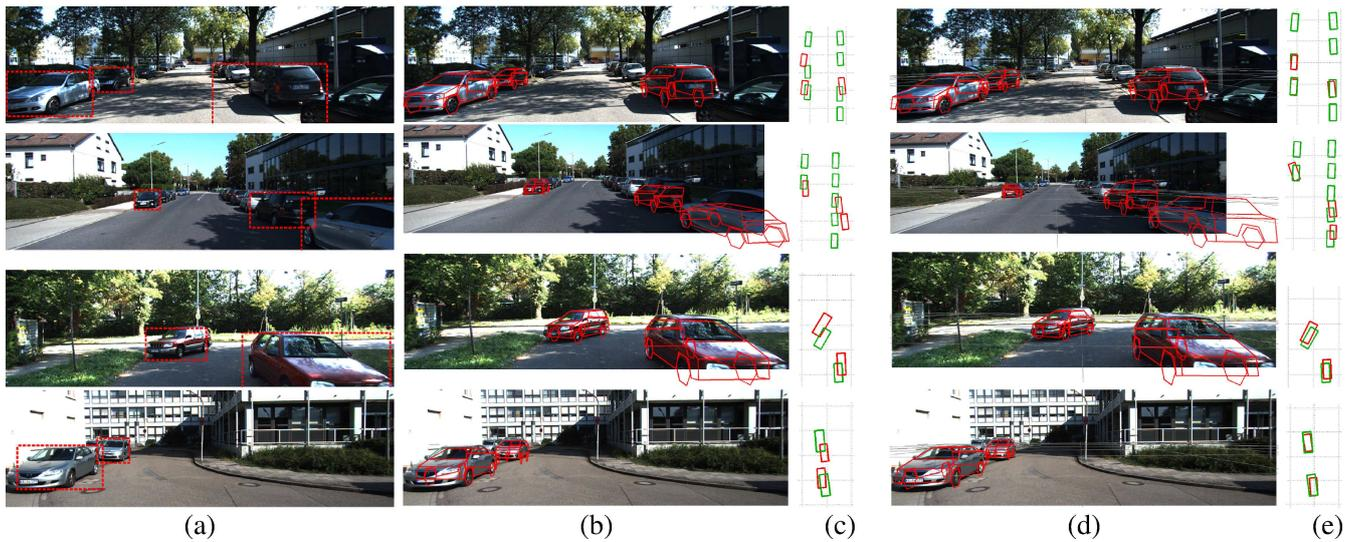
Fig. 10: FG (a-c) vs FG+GP (d,e). (a) 2D bounding box detections, (b) FG based on (a), (c) bird's eye view of (b), (d) FG+GP shape model fits, (e) bird's eye view of (d). Estimates in red, ground truth in green.
