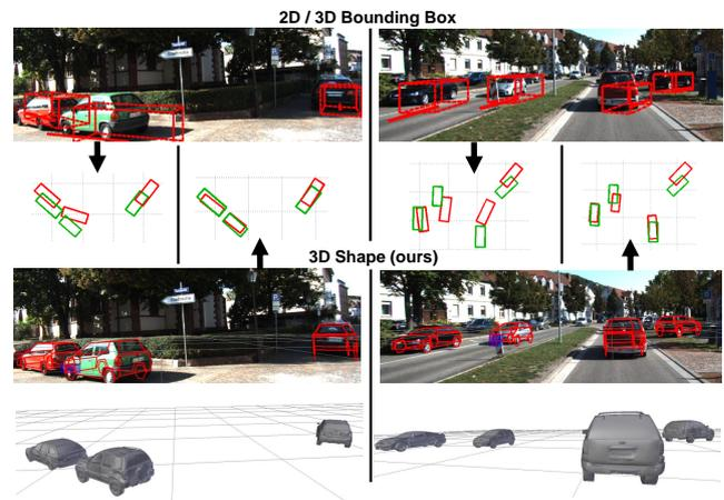
Fig. 1: *Top*: Coarse 3D object bounding boxes derived from 2D bounding box detections (not shown). *Bottom*: our fine-grained 3D shape model fits improve 3D localization (see bird's eye views).
