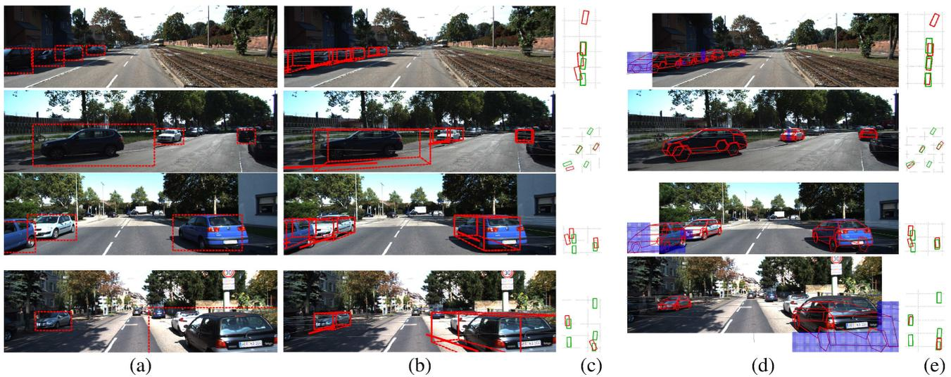
Fig. 8: COARSE+GP (a-c) vs FG+GP+DO+SO (d,e). (a) 2D bounding box detections, (b) COARSE+GP based on (a), (c) bird's eye view of (b), (d) FG+GP+DO+SO shape model fits (blue: estimated occlusion masks), (e) bird's eye view of (d). Estimates in red, ground truth in green.
