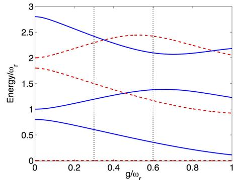
FIG. 2. **Spectrum of the quantum Rabi model.** Energy levels of the quantum Rabi model as a function of the dimensionless parameter  $g/\omega_r$ . We assume  $\hbar = 1$ . Parameter values are expressed in units of  $\omega_r$  and we consider a detuned system qubit  $\omega/\omega_r = 0.8$ . Energies are rescaled in order to set the ground level to zero. The parity of the corresponding eigenstates is identified, blue continuous line for odd and red dashed lines for even states.
