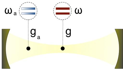
FIG. 1. **Sketch of a hypothetical quantum-optical implementation of the proposed system.** A single-mode quantum optical cavity interacts with a qubit (red, solid color) of frequency  $\omega$  in the ultra-strong coupling regime. The coupling  $g$  is of the same order of the qubit and resonator frequencies. Another qubit (blue, shaded color) can be used as an ancillary system in order to measure and manipulate USC polariton states.
