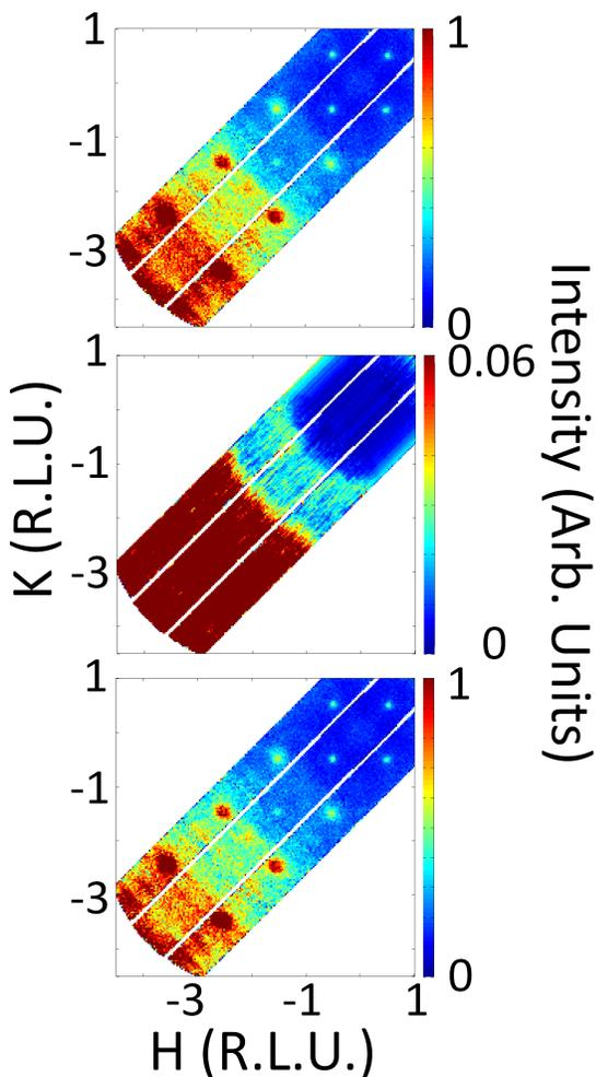
FIG. S2.  $HK$  maps produced identically to Fig. 2 of the main manuscript. a) A normalized signal data set with no empty can subtraction is shown. b) A normalized empty sample can data set on an intensity scale 6% of that of either a) or c) is shown. c) A normalized signal minus background data set is shown on the same intensity scale as in a). This is the same data as presented in Fig. 2 of the main manuscript. All data sets shown were collected at 7 K.
