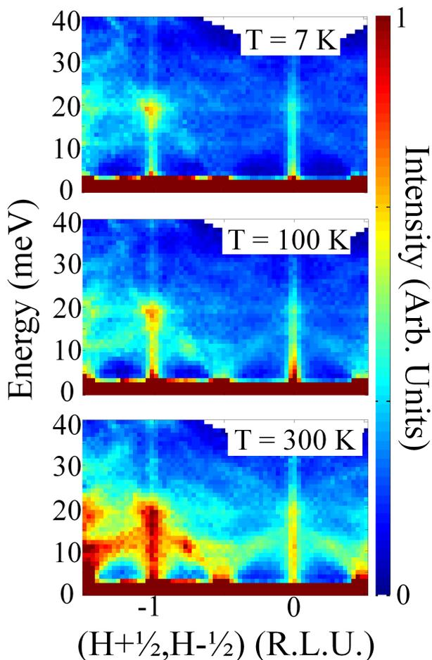
FIG. 4. Energy vs. Wave-vector maps at a) 7, b) 100 and c) 300 K.  $L$  has been integrated from  $-4$  to  $4$  and  $HH$  has been integrated from  $0.4$  to  $0.6$ , as in Fig. 1.
