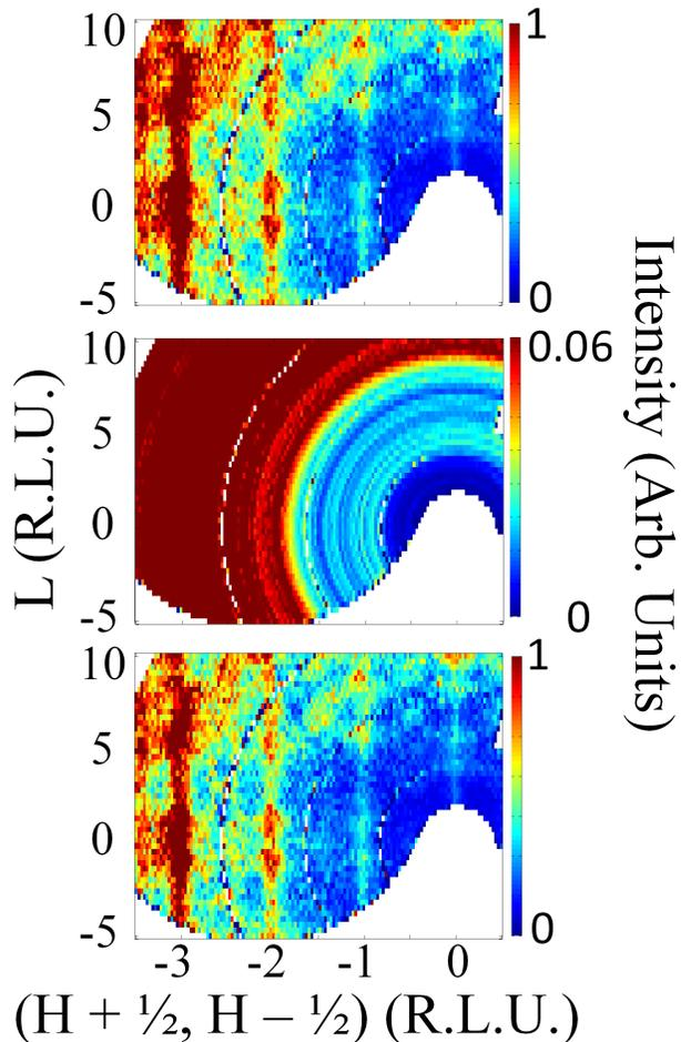
FIG. S3.  $HHL$  maps produced identically to Fig. 3 of the main manuscript. a) A normalized signal data set with no empty can subtraction is shown. b) A normalized empty sample can data set on an intensity scale 6% of that of either a) or c) is shown. c) A normalized signal minus background data set is shown on the same intensity scale as in a). This is the same data as presented in Fig. 3 of the main manuscript. All data sets shown were collected at 7 K.
