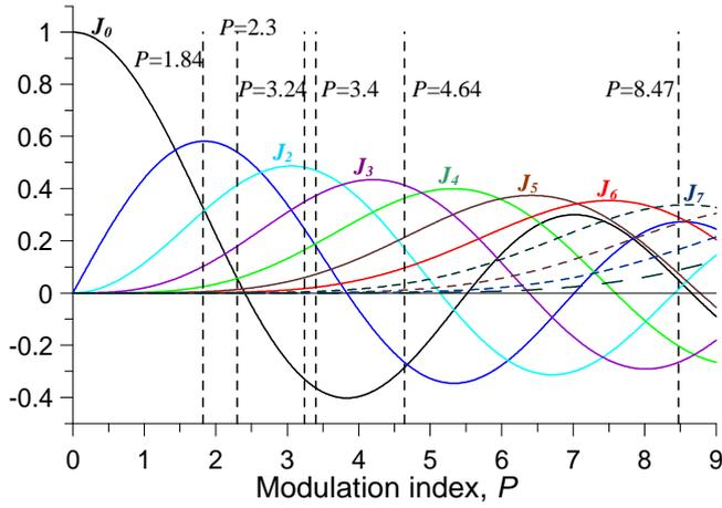
Fig. 1. (Color online) Bessel functions from  $J_0(P)$  up to  $J_{10}(P)$  versus modulation index,  $P$ . The dashed not labeled lines starting up from zero more and more gradually, correspond to  $J_8(P)$ ,  $J_9(P)$ , and  $J_{10}(P)$ , respectively. Amplitudes and initial phases of the respective spectral components in (5) are determined by the Bessel function order, taking into account the relation  $J_{-n} = (-1)^n J_n$
