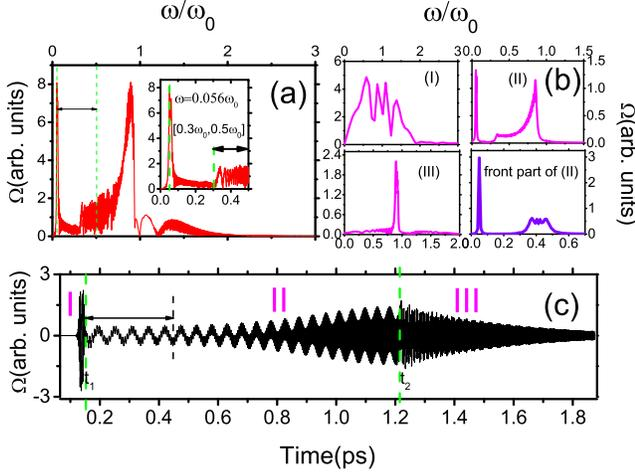
FIG. 1: Electric field profile and spectrum for three successive time regions.  $\omega_c = 0.1\text{fs}^{-1}$ ,  $A = 4\pi$ ,  $L = 150\mu\text{m}$ ,  $t_1 = 0.15\text{ps}$ ,  $t_2 = 1.2\text{ps}$ .  $[t_i, t_1]$ ,  $[t_1, t_2]$  and  $[t_2, t_f]$  are labeled by I, II and III respectively. The below insets are the corresponding spectrums for those three regions, while the above inset is the spectrum of the first five oscillations in region II.
