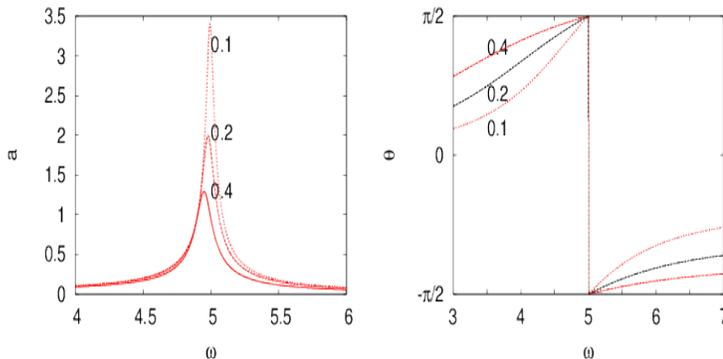
FIG. 6: Plot of the amplitude  $a(\omega)$  (left panel) and the phase  $\theta(\omega)$  (right panel) for three different values of the coupling  $\kappa = 0.4, 0.2$  and  $0.1$ . The other parameters are  $\omega_r = 5, \alpha = 0.01$ .
