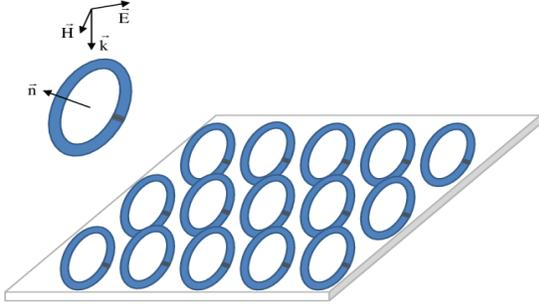
FIG. 1: Schematic view of the electromagnetic wave incident on the layer containing split ring Josephson junction resonators. One ring is shown, indicating the orientation.
