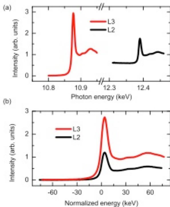
**S3 | X-ray near edge absorption spectroscopy (XANES) measurements investigating SOC. a** XANES results at the L<sub>2</sub> and L<sub>3</sub> absorption edges for NaOsO<sub>3</sub>. **b** The XAS results shifted in energy to be centered at zero on their respective absorption energies and the intensities normalized to allow a comparison. The ratio of the integrated intensities is 2.6:1.
