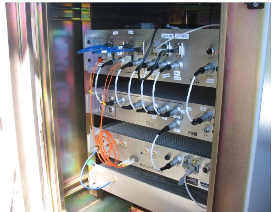
Figure 5. The RF-shielded rack housing BIGHORNS back-end components (from the bottom to top : box with a second gain stage and RF-filters; BEDLAM spectrometer; power unit; and PC computer unit).
