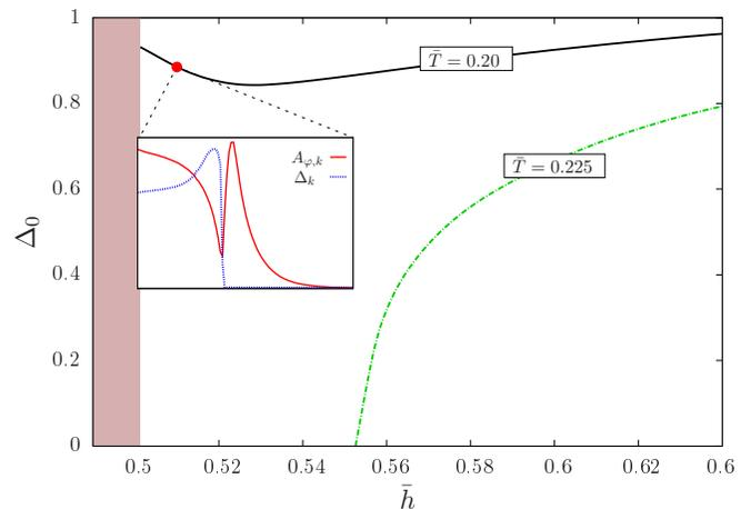
Figure 7. Fermion gap for two different values of  $\bar{T}$  and fixed  $\bar{m} = 0.74$  (corresponding to a Li-K mixture) as a function of  $\bar{h}$ . The red/dark-shaded area indicates the regime where  $A_{\varphi,k} \rightarrow 0$  for  $\bar{T} = 0.20$ . The inset shows the  $k$ -evolution of  $A_{\varphi,k}$  and  $\Delta_k$  for  $(\bar{T}, \bar{h}) = (0.20, 0.51)$ .
