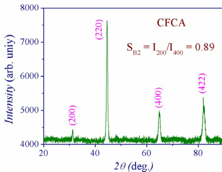
FIG. 2. Powder x-ray diffraction pattern of CFCA at room temperature.
