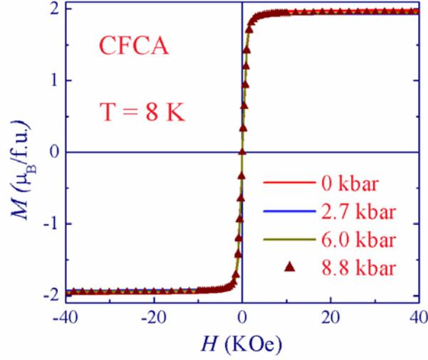
FIG. 3. Isothermal magnetization curves of CFCA obtained under various applied hydrostatic pressures at 8 K.
