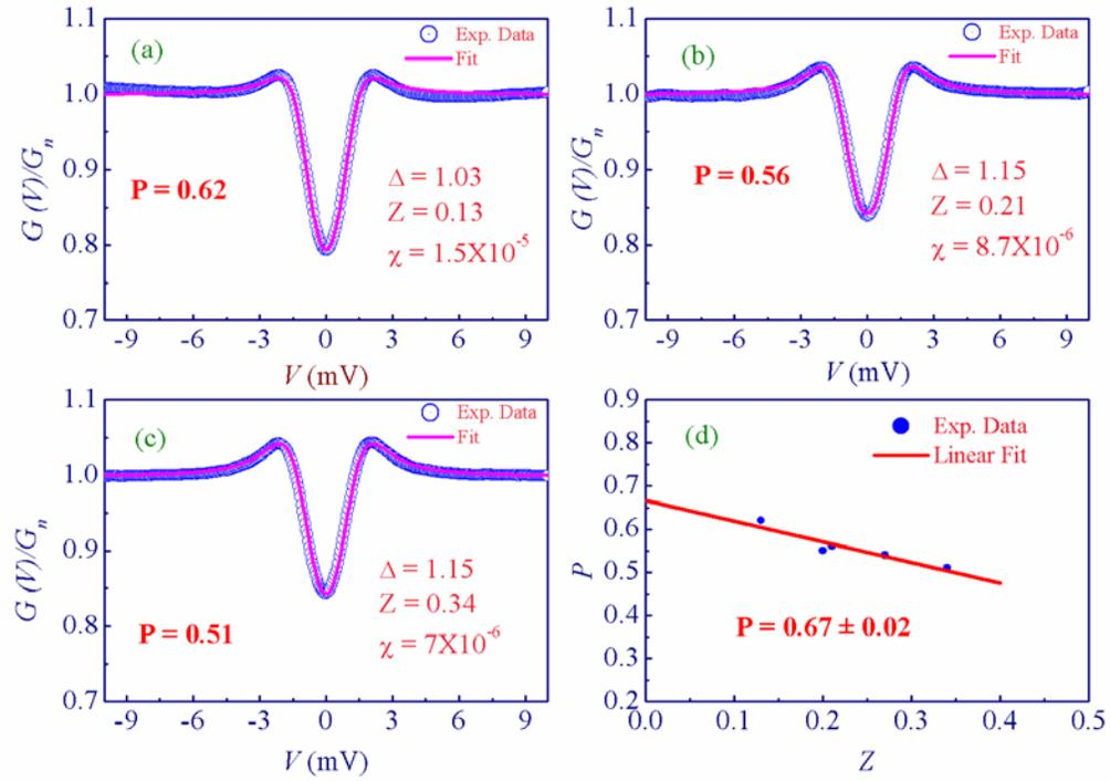
FIG. 4. (a) – (c) Normalized conductance curves of CFCA obtained at 4.2 K. The open circles denote the experimental data and the solid lines are the fit to the data using modified BTK model. (d) P vs. Z curve with the linear fit.
