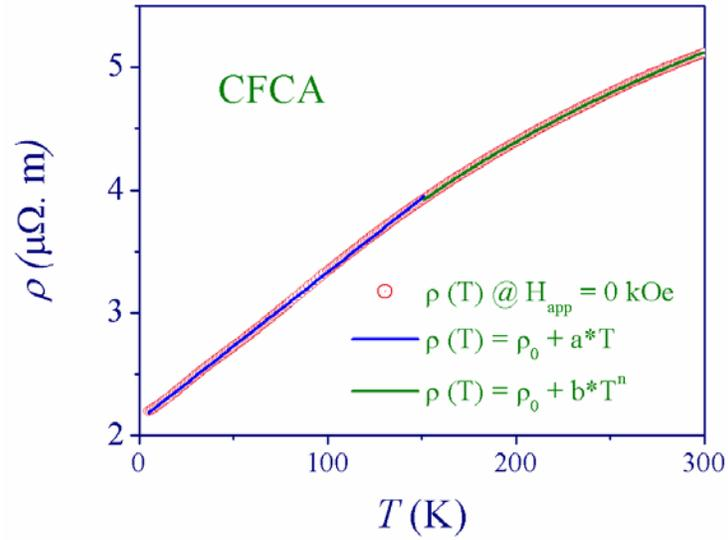
FIG. 5. Electrical resistivity variation with temperature of CFCA in the range of 5-300 K. The open circles denote the experimental data and the solid lines are the fit to the data to the equation  $\rho(T) = \rho_0 + a \cdot T$  in the low temperature regime (5-150 K) and  $\rho(T) = \rho_0 + b \cdot T^n$  in the range of 150-300 K.
