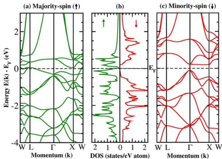
FIG. 1. Band structure and density of states of CFCA: (a) majority-spin bands, (b) density of states, (c) minority-spin bands at experimental lattice parameter ( $a_{\text{expt}} = 5.75 \text{ \AA}$ ).
