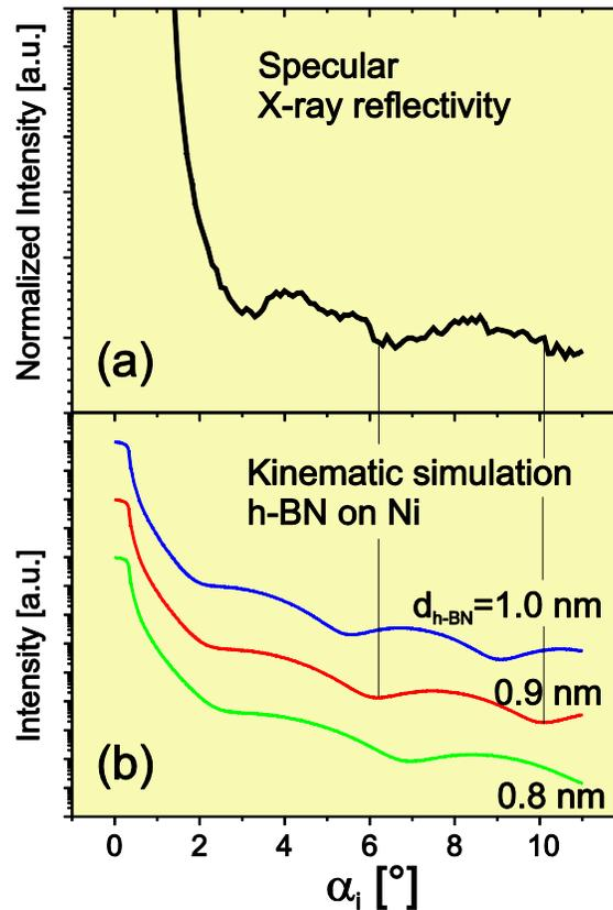
Figure 3. (a) Experimentally observed specularly reflected x-ray intensity collected from a continuous h-BN film on Ni synthesized at 730 °C over 5 hours. (b) Kinematic scattering simulations for a h-BN layer with the thickness ( $d_{\text{h-BN}}$ ) varying between 0.8 and 1.0 nm on a Ni substrate.
