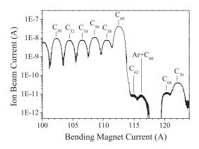
FIG. 2. Beam spectrum of extracted ions from the mixture plasma of  $C_{60}$  and Ar in the ECRIS.
