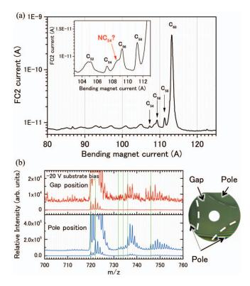
FIG. 3. (a) Beam spectrum of extracted ions and (b) LDI-TOF-MS spectra of the deposited material on the plasma electrode (substrate) of the gap and pole positions, obtained with -20 V bias voltage. The right-side photo shows the irradiated substrate on which materials were deposited. The gap and pole positions correspond to the region, respectively, inside or outside the triangular mark.
