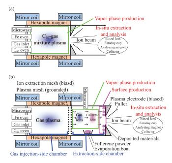
FIG. 1. Schematic drawings of (a) one-chamber and (b) two-chambers configurations of the Bio-Nano ECRIS.
