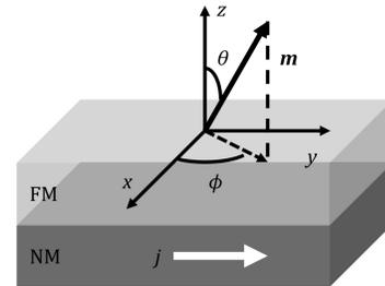
FIG. 1. Schematic diagram of the bilayer spin Hall effect device. Electric current  $j$  flows along the  $y$  axis.
