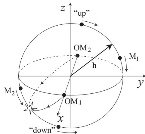
FIG. 4. Equilibrium states shown as points on the unit sphere for small  $\alpha_j > 0$  in the absence of external field. Arrows show the directions of equilibria displacements as an external field  $\mathbf{h}$  is increased at constant  $\alpha_j$ . Points  $OM_1$ ,  $OM_2$ , and  $S_2$  eventually merge into  $X$ .
