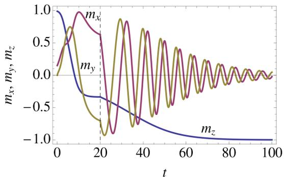
FIG. 9. (color online) Evolution of the three components of the magnetization in a two stage switching process. The parameters are:  $h_y = 0.15$ ,  $\alpha_j = 0.45$ , and  $\alpha = 0.05$ . The field-current pulse is turned on at  $t = 0$  and off at  $t = 20$ .
