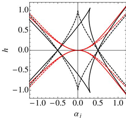
FIG. 7. (color online) Tilted current-field phase diagram at  $\alpha = 0$ . The black and red(gray) lines correspond to  $h_{cM}$  and  $h_{cOM}$ , respectively. The solid lines represent the diagrams with a tilting angle of the field set to be 15 degree with respect to  $\hat{y}$  direction. The dashed lines represent the diagram with  $\mathbf{h} \parallel \hat{y}$ . Opposite tilting happens when the angle is negative.
