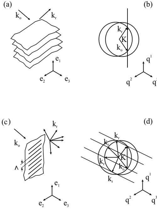
FIG. 1: Translation-invariant sets and reciprocal gratings for optical diffraction from three-dimensional (a, b) and two-dimensional (c, d) holographic gratings: (a, c) - the coordinate space, (b, d) - the  $k$ -space;  $\mathbf{K}$  is the scattering vector (shown only for scattering “forward”),  $\mathbf{k}_0$  and  $\mathbf{k}_r$  are the wave vectors of the readout and reconstructed beams, respectively,  $\Lambda = 2\pi/K$  is the grating period.
