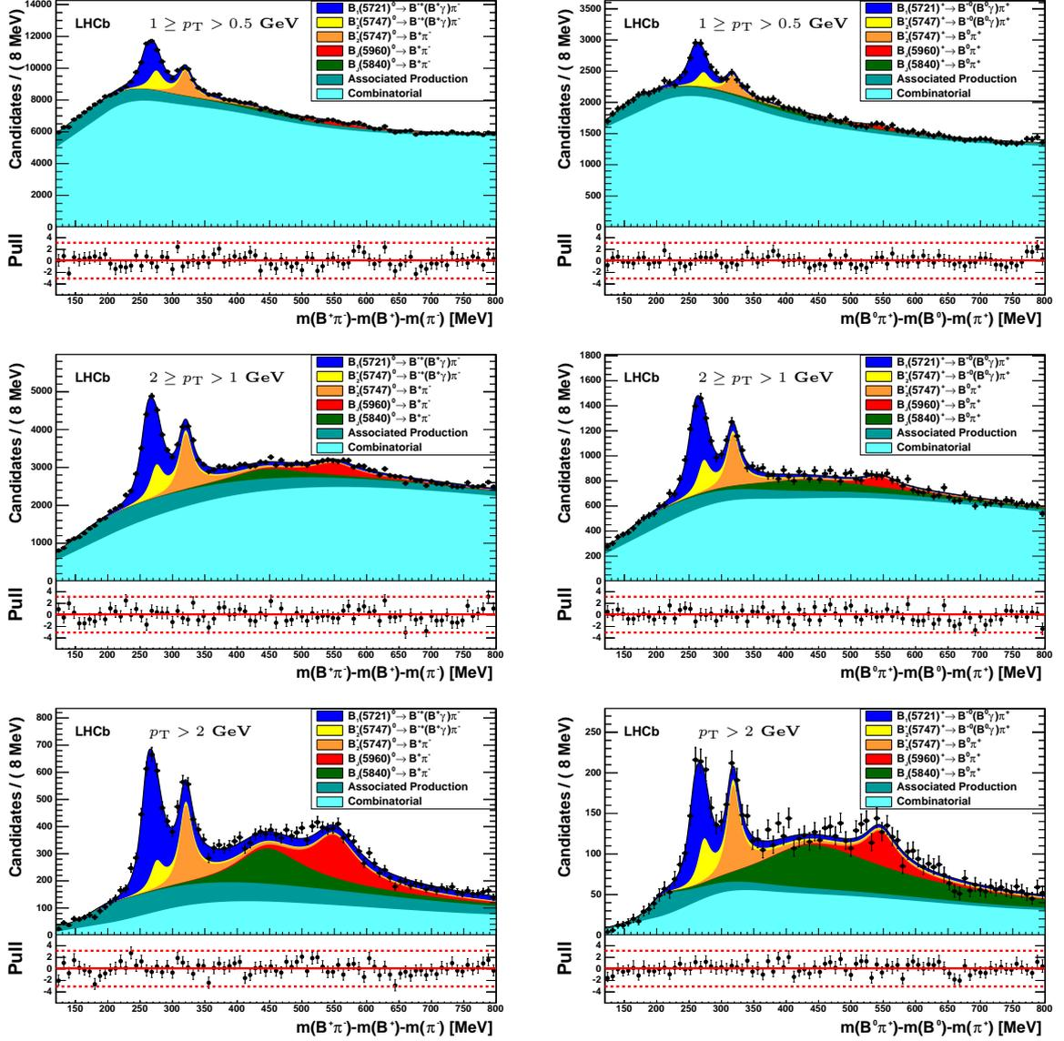
Figure 5: Result of the fit to (left)  $B^+\pi^-$  and (right)  $B^0\pi^+$  candidates, split into (top to bottom) low, medium and high  $p_T$  bins, with ranges as labelled on the plots. The components are labelled in the legends. The fit pulls are shown underneath each plot.
