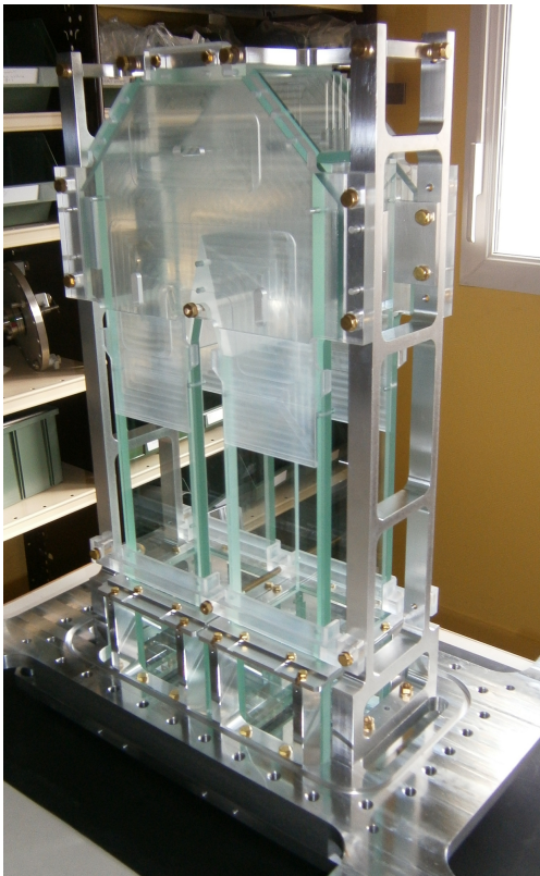
Figure 5. Bare float-glass structure held by the aluminium and PMMA support.
