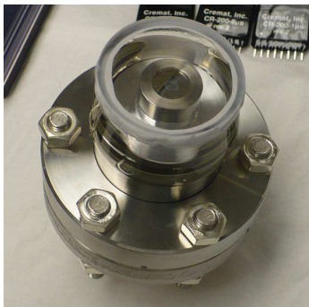
Fig. 3. The custom-built xenon scintillation source.
