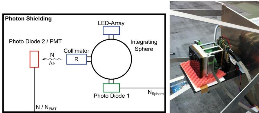
**Figure 4.** Left: Sketch of the calibration stand for photo sensors. Right: first fully assembled Photo Detector Module (PDM) for JEM-EUSO prototype experiments.
