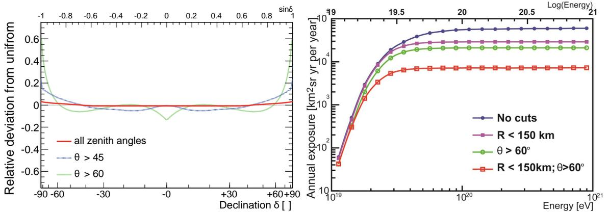
**Figure 6.** Left: Relative deviation from uniformity of the aperture as a function of sine of declination. The curves show the cases for a selection of events with different zenith angle. Right: Annual exposure of JEM-EUSO (ISS at 400 km) for the full FoV and for the case of extremely high quality cuts applied to the data. For the most stringent cuts, the threshold is low enough for an overlap with ground based experiments with good statistics. Plots adapted from [9].
