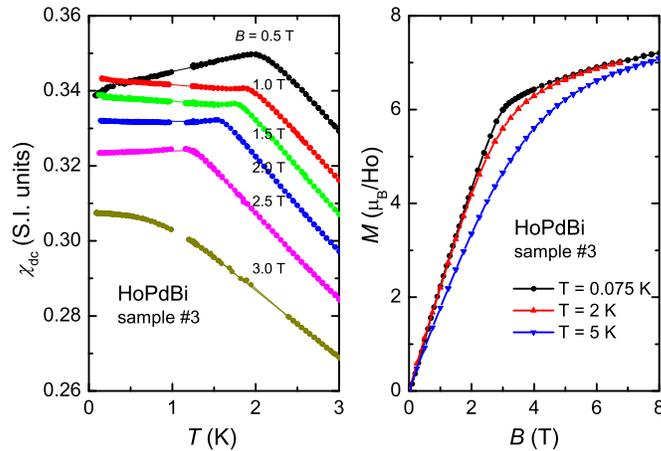
**Figure 4.** Left panel: Magnetic susceptibility of HoPdBi sample #3 as a function of temperature measured in magnetic fields up to 3 T as indicated. Right panel: Magnetization in fields up to 8 T at temperatures of 0.075, 2.0 and 5.0 K.
