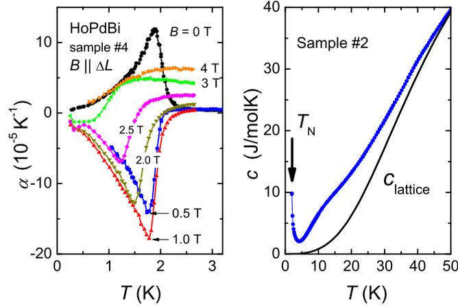
**Figure 5.** Left panel: Coefficient of linear thermal expansion as a function of temperature of HoPdBi (sample #4) measured in zero and applied fields as indicated. Right panel: Specific heat (sample #2) in a plot of  $c$  versus  $T$  up to 50 K. The solid line indicates the lattice contribution given by the Debye function with  $\theta_D = 193$  K.
