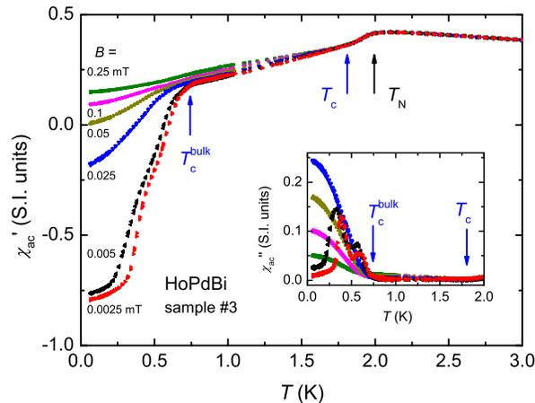
**Figure 3.** Real part of the ac-susceptibility of HoPdBi sample #3 for driving fields of 0.0025, 0.005, 0.025, 0.05, 0.10 and 0.25 mT, from bottom to top. Arrows indicate  $T_N$ ,  $T_c$  and  $T_c^{bulk}$ . The inset shows the corresponding imaginary part of  $\chi_{ac}$ .
