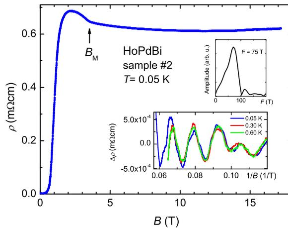
**Figure 6.** Resistance of HoPdBi sample #2 as a function of the magnetic field at  $T = 0.05$  K. The arrow indicates the antiferromagnetic phase boundary at  $B_M$ . Lower inset:  $\Delta\rho$  as a function of  $1/B$  showing the Shubnikov - de Haas effect at 0.05, 0.3 and 0.6 K. Upper inset: fast Fourier transform of the data with frequency  $F = 75 \pm 5$  T.
