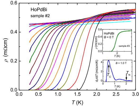
**Figure 2.** Resistivity as a function of temperature for HoPdBi sample #2 measured in fixed magnetic fields: from right to left 0 T to 1.1 T in steps of 0.1 T, 1.2 T to 2 T in steps of 0.2 T, and 2.25 T, 2.5 T and 3 T. Lower inset: Derivative  $d\rho/dT$  versus  $T$  for  $B = 1.0$  T; arrows indicate  $T_C$  and  $T_N$ . Upper inset:  $\rho(T)$  versus  $T$  in zero field for sample #3.
