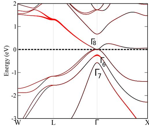
**Figure 8.** Calculated bulk band structure of the half-Heusler HoPdBi. The projection of the Pd- $s$  states is highlighted by the size of the filled red circles. Bands  $\Gamma_{6,7,8}$  are labeled according to the symmetry of their wave functions. The Fermi energy,  $E_F$ , is shifted to zero (horizontal dashed line). The measured sample is slightly  $p$ -doped, which will cause  $E_F$  to lie marginally below zero.
