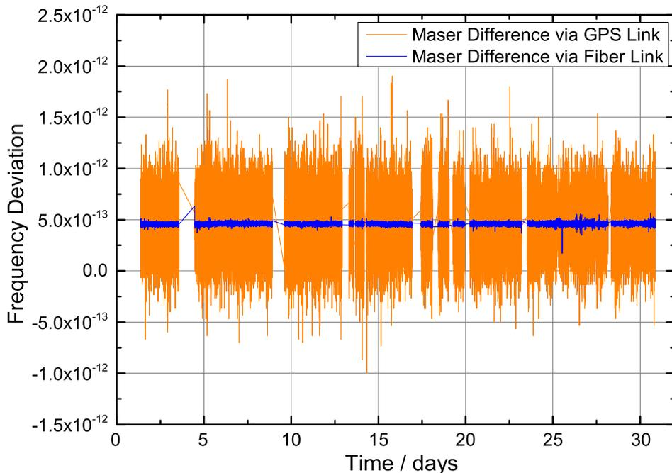
**Figure 5.** Frequency deviation between the two masers at MPQ and PTB measured over the GPS link and over the fiber link, respectively. The masers show a mean frequency difference of about  $4.6 \times 10^{-13}$  with respect to each other. The occasional gaps in the fiber link data are due to cycle-slips and a malfunction of one of the frequency comb systems. GPS link data are only shown at intervals when the fiber link data were available.
