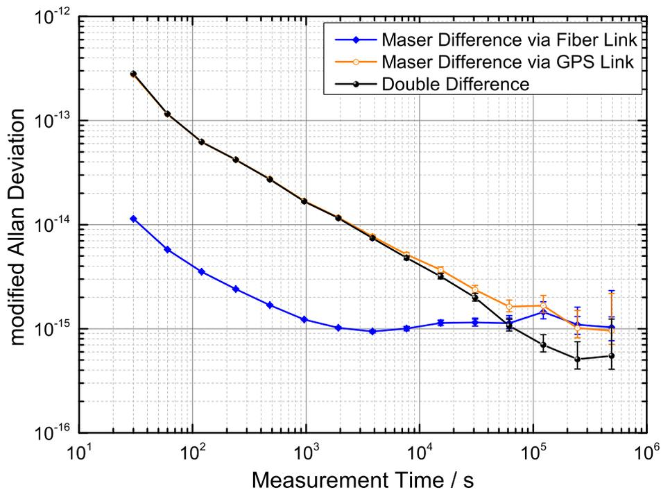
**Figure 4.** Frequency instability of the maser difference measured via the fiber link and via the GPS link, respectively. The double difference reveals the true GPS link performance without any contribution from the masers.
