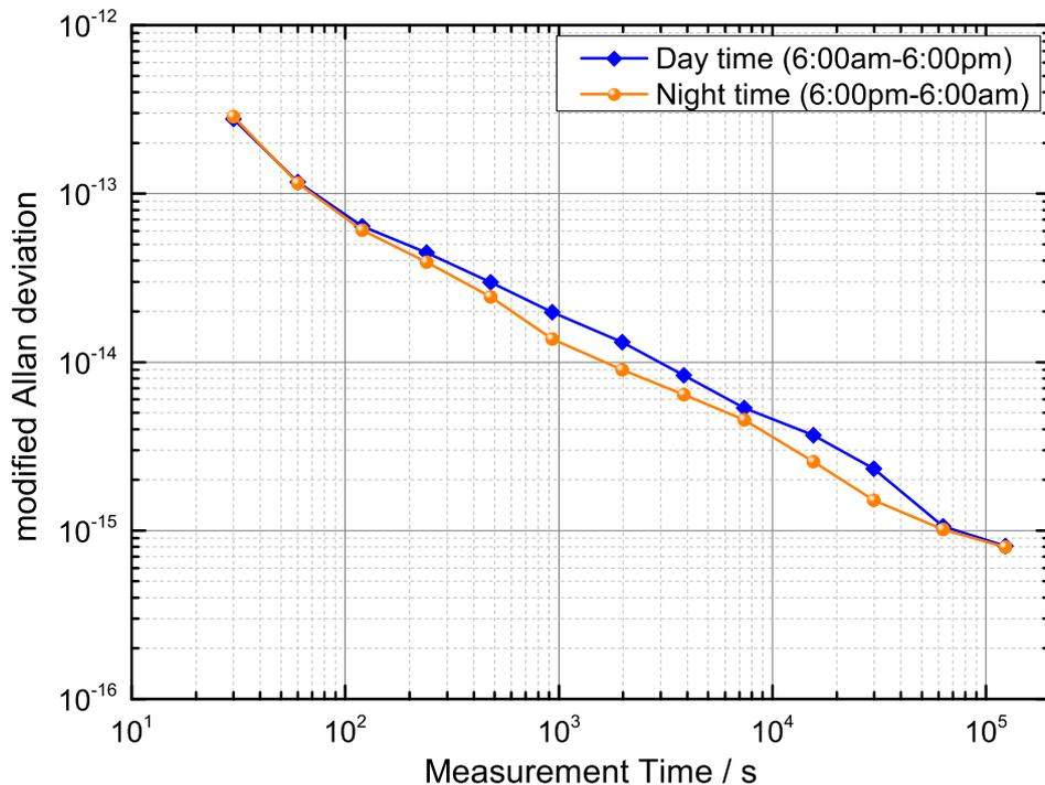
**Figure 6.** Frequency instability of the double difference for the day time from 6:00 am to 6:00 pm and for the night time from 6:00 pm to 6:00 am.
