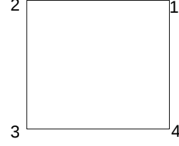
FIG. 4. Labeling of the four sublattices is as shown in the square. The labeling of the four Dirac points in Brillouin zone also follows the same numbering.
