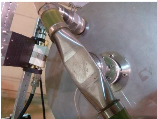
Fig. 9: Picture of the prototype installed at the FNG neutron source.
