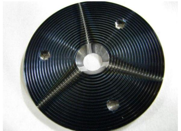
Fig.17. Sputtering marks at the extraction electrode of KVI AECRIS.
