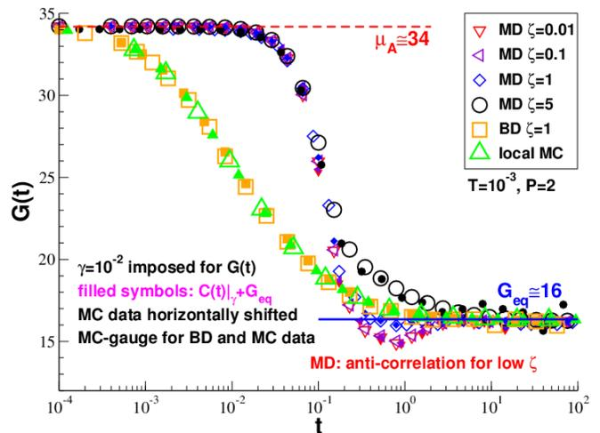
FIG. 4: Stress relaxation modulus  $G(t)$  (open symbols) and rescaled autocorrelation function  $C(t)|_\gamma + G_{\text{eq}}$  (filled symbols) for MD simulations for several friction constants  $\zeta$ , BD simulations with  $\zeta = 1$  and local MC moves. Shifting horizontally the MC data by a factor  $1/8000$  allows to bring them to collapse onto the BD data.
