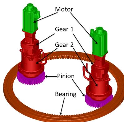
**Figure 2:** Azimuth drive sub-assembly.
