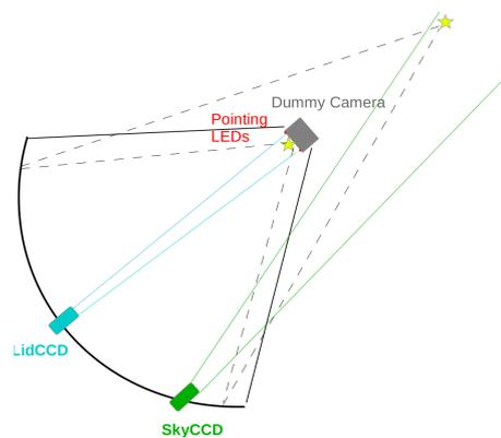
**Figure 5:** Sketch of the 2 CCD camera pointing setup.
