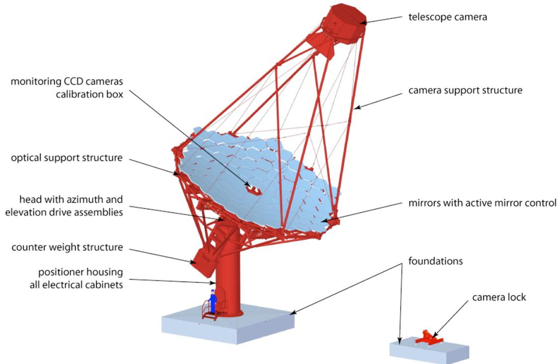
**Figure 1:** Illustrative description of the MST design with the main components.
