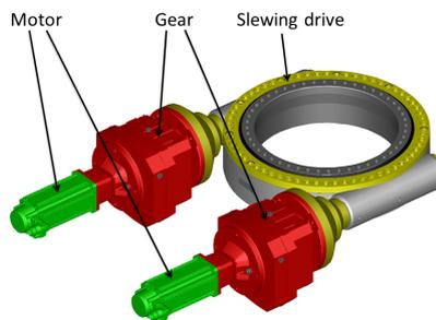
**Figure 3:** One of the two elevation drive sub-assemblies.
