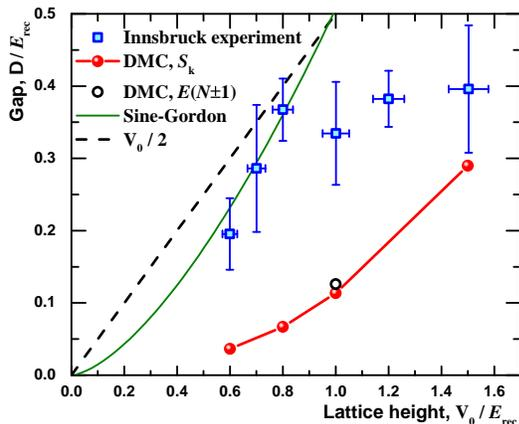
FIG. 5: (Color online) Energy gap. Squares with error bars, experimental data from Ref. [24]; filled circles, DMC prediction obtained from the fit to  $S(k \rightarrow 0)$ ; open circle, DMC prediction obtained according to Eq. (7); solid line, sine-Gordon model [24]; dashed line, upper bound given by  $V_0/2$ .  $a_{1D}/a_0 = 0.18182$ .
