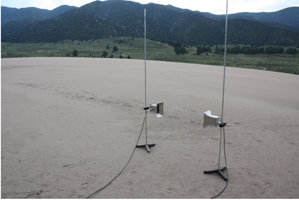
FIG. 12: The two horn antennas used for the Great Sand Dunes National Park experiment, in a near-surface setup.
