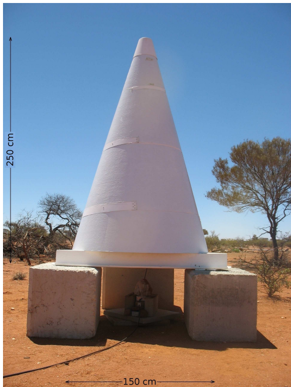
Figure 1. The conical log-spiral antenna as deployed at the MRO in October 2014. The antenna was painted in order to protect the copper conductor from the weather.
