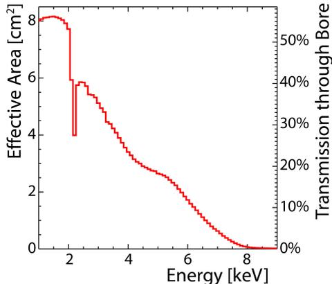
**Figure 3.** Effective area ( $\text{cm}^2$ ) and transmission (percentage) versus energy. The transmission is computed by dividing the effective area (EA) by the geometric area of the 43 mm diameter bore. The EA was modelled using the as-built optical prescription, assuming a half-power diameter of 75 arcsec and that the solar axion emission comes from a uniformly distributed 3 arcmin disc.
