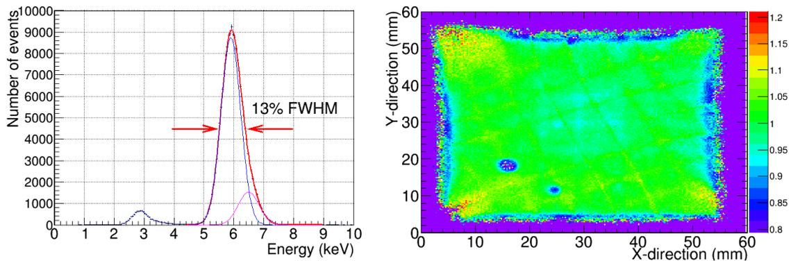
**Figure 6.** Left:  $^{55}\text{Fe}$  calibration spectrum of the sunrise Micromegas detector. The main peak has been fitted to two gaussian functions (blue and magenta lines, in red the sum of them), corresponding to the  $K_\alpha$  (5.9 keV) and  $K_\beta$  lines (6.4 keV). Right: Gain uniformity of the sunrise Micromegas detector. The dead areas (in purple) show lower values than unity (in green) and lie outside the axion signal area.
