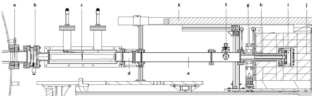
**Figure 1.** Sketch of the new CAST sunrise detection line composed of a low background Micromegas detector placed at the focal point of an x-ray optic. The different parts of the line are described in detail in the text: gate valve (a), differential window (b), Wolter I x-ray optic (c), bellow (d), stainless steel interface tube (e), calibration system (f), precision stage (g), copper interface tube (h), Micromegas detector (i), lead shielding (j) and muon veto (k).
