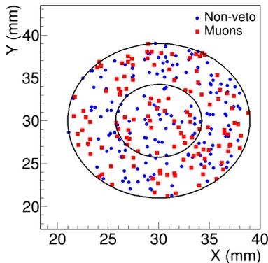
**Figure 16.** A 2D hitmap of background events in the calibration area (outer circle) with energies between 2 and 14 keV, where the two populations of muon-induced events (muons) and the rest (non-veto) are indicated in red and blue respectively. The inner circle marks the position of the cathode window opening, which includes the spot.
