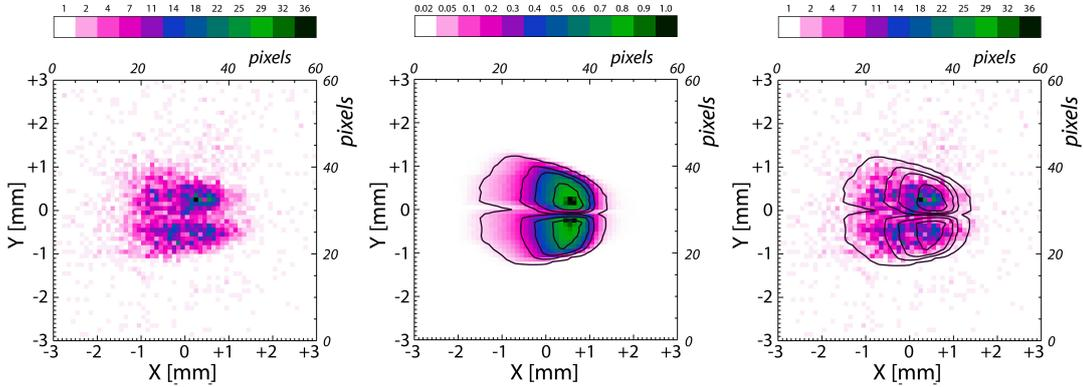
**Figure 12.** Cool-X x-ray source illumination of the new x-ray telescope. Left: image measured by the Micromegas detector. Middle: simulation, assuming the Cool-X x-ray emission comes from a uniform 6 mm diameter spot. Contour levels are 6%, 30%, 50% and 80% of maximum intensity. Right: data of the Micromegas detector, now with the simulation contours over-plotted.
