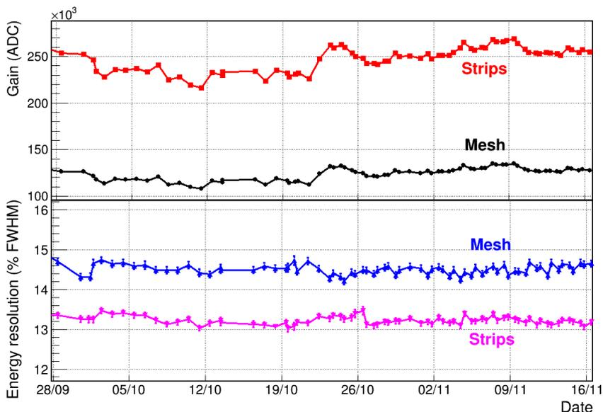
**Figure 15.** Evolution of the gain and the energy resolution (%FWHM at 5.9 keV) of the detector during the data-taking. The fluctuations, measured both at the mesh and at the strips are less than 5%.
