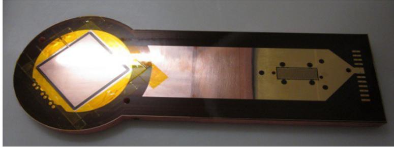
**Figure 5.** A photograph of the new sunrise Micromegas readout glued on the copper support. At the left of the image is the squared active area, while the strip signals are extracted from a central connector situated on the right part. The high voltage is fed through squared pads situated on the right part and reach the mesh and the field shaper through lines situated at the sides of the printed board.
