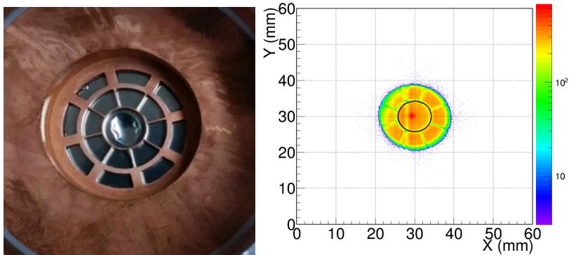
**Figure 8.** Left: Photo of the new copper strongback with the spider web design. Right: Intensity plot with the projection of the x-ray window (cathode) in the Micromegas detector during the calibrations.
