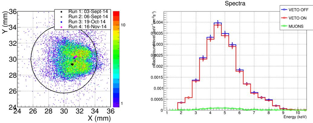
**Figure 14.** Left: Intensity map of the calibration with the x-ray finger through the x-ray optic. The outer contour is the region used (conservatively) to define the background in the spot. Each of the four dots corresponds to the centroid of a spot-calibration with the x-ray finger. Their statistical error are within the dot size. Right: Energy spectrum of an x-ray finger run. The higher end of the spectrum is reduced because of the focusing optic’s efficiency loss at these energies.
