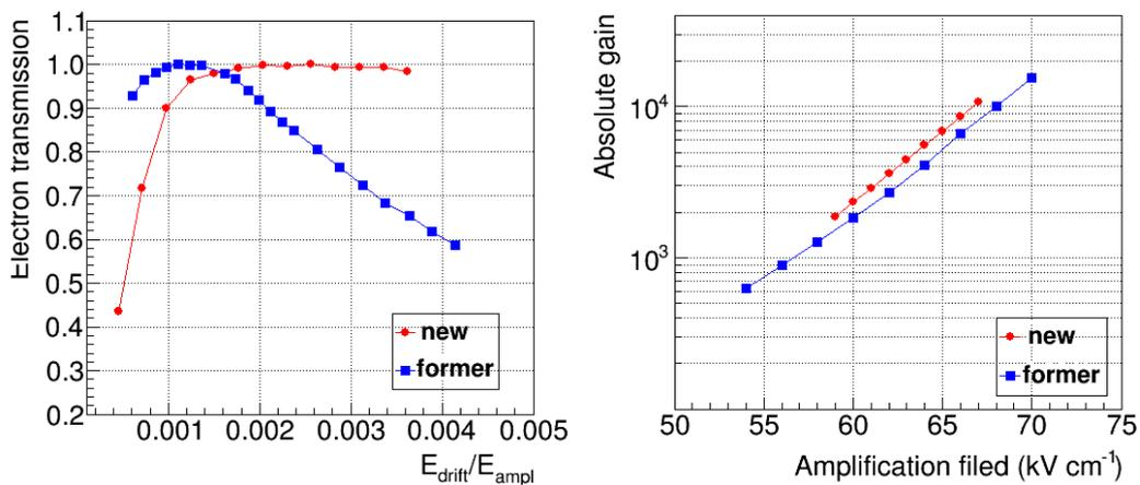
**Figure 7.** Dependence of the electron transmission on the ratio of drift and amplification fields (left) and of the absolute gain on the amplification field (right) for a new CAST sunrise Micromegas detector (circled red line) and a former design (squared blue line), characterized in  $\text{Ar}+2\%\text{iC}_4\text{H}_{10}$  at 1.4 bar.
