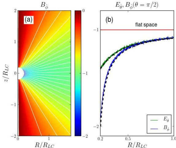
FIG. 2.— Monopole test with GR PIC. Electromagnetic fields are normalized to  $(r/R_{LC})B_{\hat{r}}$ . (Panel a): Poloidal field lines are shown as white, color represents toroidal field  $B_{\hat{\phi}}$ . (Panel b): Slice of  $B_{\hat{\phi}}$  and  $E_{\hat{\theta}}$  at the equator. Black dashed lines show analytical estimates of  $B_{\hat{\phi}}$  (14) and  $E_{\hat{\theta}}$  (15). Red solid line represents flat spacetime solution  $E_{\hat{\theta}} = B_{\hat{\phi}}$ .
