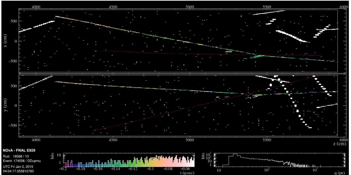
Figure 4: In this event, a slightly downward-going muon, likely originating from a cosmic ray interaction outside the detector, enters from the high-z extreme of the detector, scatters upward within it, and produces an upward-going track.
