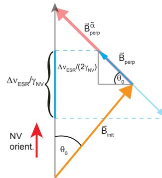
FIG. 8: Detailed, two-dimensional view of the schematic presented in Fig. 7c. The figure illustrates how misalignment angle  $\theta_0$  and perpendicular field strength  $|B_{\text{perp}}^{\tilde{\alpha}}|$  can be determined from the dataset in Fig. 7d, in order to compensate the initial misalignment in magnetic field.
