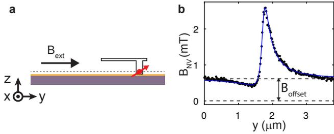
FIG. 5: The external B-field  $B_{\text{ext}}$  (a) causes a  $B_{\text{offset}}$  in the measured field (b), allowing to detect negativ B-field projections.
