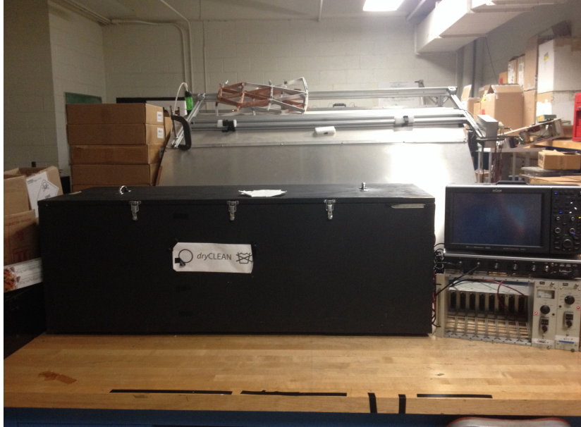
Figure 3: The dark box and oscilloscope used in the SPE characterization setup. The dark box is lined with magnetic shielding and covered with felt on both the inside and outside to prevent reflections and light leaks. The oscilloscope is a LeCroy WaveRunner 606Zi 600MHz
