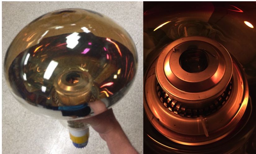
Figure 1: ETL 11-inch D784UKFL PMT prototype. In the left image, the discolored area can be seen on the center of the glass envelope. The right image shows the first dynode of the 12-stage amplifier chain.
