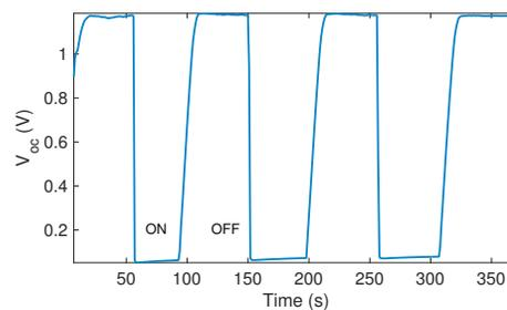
FIG. S5: Time evolution of the measured open-circuit voltage vs a Ag/AgCl reference electrode. The photo-anode consisted of Au/TiO<sub>2</sub>[50 nm]/Au. Electrolyte: 0.5M Na<sub>2</sub>SO<sub>4</sub> with 20v/v% methanol. Light source 300 W Xenon lamp (Newport Model no. 669092) using a  $\geq 495$  nm cut-off filter (Thorlabs FGL-495).
