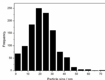
FIG. S1: Measured size distribution of the Au nanoparticles.
