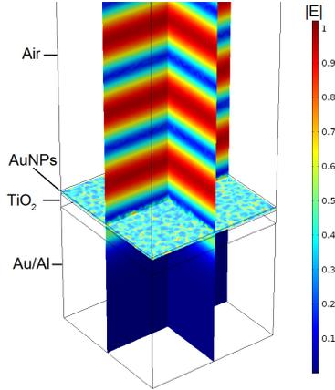
FIG. S6: The FEM model geometry used to calculate the total absorption of the device and the location of the absorption. Here the normalized magnitude of the electric field is shown.
