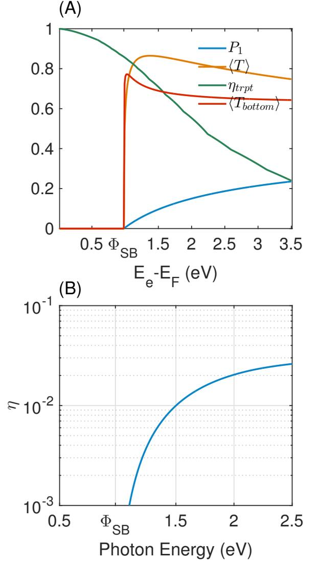
FIG. S10: Internal quantum efficiency. (A) Plots of  $\eta_{trpt}$  and  $\eta_{inj}$  shown as a function of electron excess energy above the metal’s Fermi level ( $E_F$ , in eV). For comparison, we also reproduce the curves  $P_1$  and  $\langle T \rangle$  of figure S10. (B)  $\eta$  vs incident photon energy for  $\Phi_{SB}=0.98$  eV
