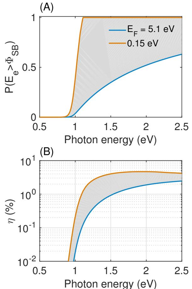
FIG. 5: **Narrow distribution of states near the Fermi level of the metal.** (A) Distribution of electron energies and (B) calculated internal quantum efficiency. The shaded areas highlight the attainable differences.  $\Phi_{SB} = 0.98$  eV.
