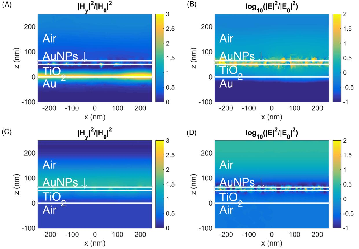
FIG. S8: spatial distribution of electromagnetic fields in samples with (A,B) and without (C,D) a metal reflecting layer for a wavelength of 600 nm.
