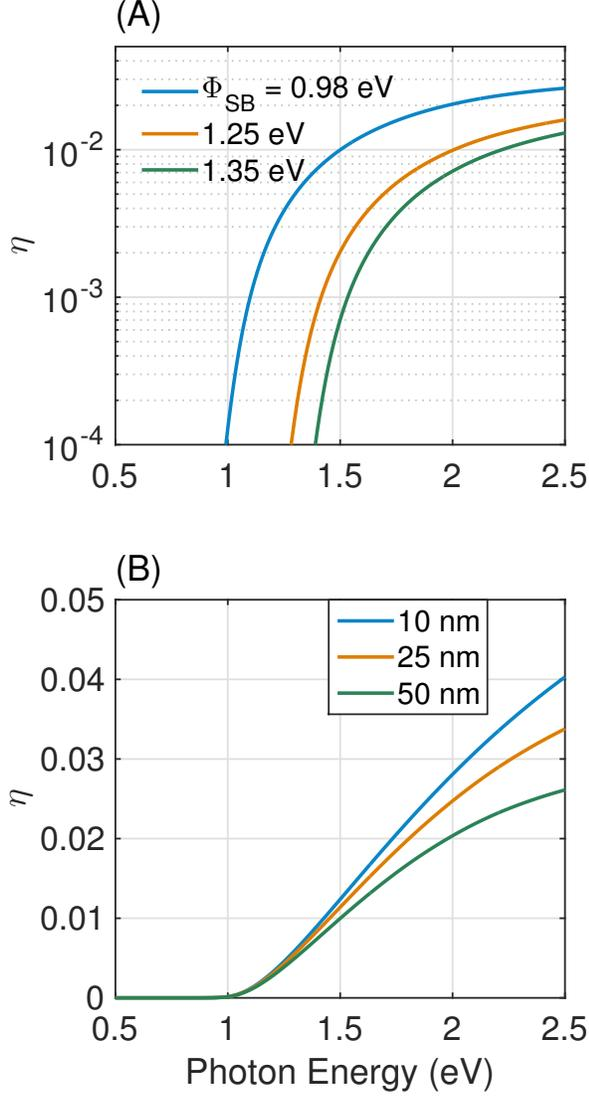
FIG. S11: Effect of Schottky barrier height (A) and semiconductor thickness (B) on  $\eta$
