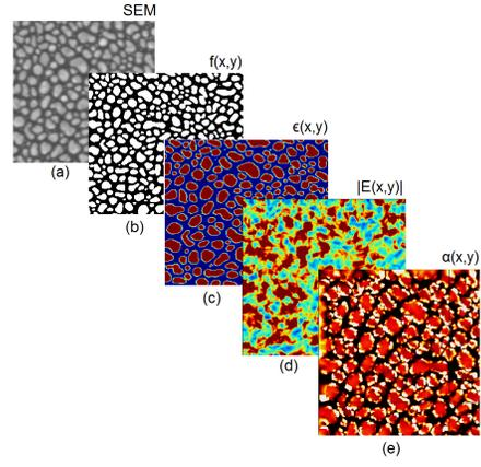
FIG. S7: A scheme for calculating absorption from SEM image. Convert the SEM (a) into a monochrome bitmap (b), then use this to define a material with  $(x, y)$ , a spatially dependent relative permittivity, (c). This material can then be used in FEM calculations to determine the electric field (d) and thus the electromagnetic absorption,  $\alpha$ , in the layer (e).
