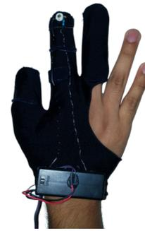
**Figure 6. Final version of Fingers. This version has only one LED located at the tip of the index finger.**
