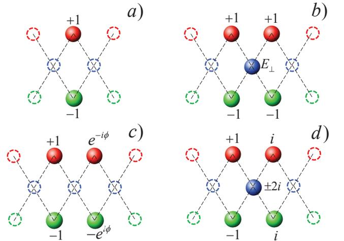
FIG. 3: CLS structure. Filled circles - excited sites with amplitudes denoted right to them. Empty circles correspond to zero amplitude. Lines indicate the hopping connections. (a)  $E_{\perp} = \phi = 0$ ,  $\lambda = 0$ ; (b)  $\phi = 0$ ,  $\lambda = 0$ ; (c)  $E_{\perp} = 0$ ,  $\lambda = 0$ ; (d)  $E_{\perp} = 0$ ,  $\phi = \pi/2$ ,  $\lambda = \pm 2$ .
