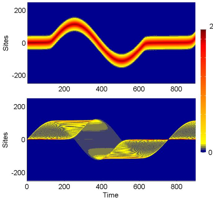
FIG. 6: The case of a gapless band structure is simulated for  $\phi = 0.1$ ,  $E_{\perp} = \sqrt{2}\sin\phi$  and  $E_{\parallel} = 0.025$ . The plots display the space-time evolution of the norm density  $\rho_n = |a_n|^2 + |b_n|^2 + |c_n|^2$ . Upper plot: initial state is Gaussian as before. Lower plot: Initial state is in the form of a single CLS as in Fig.3(a).
