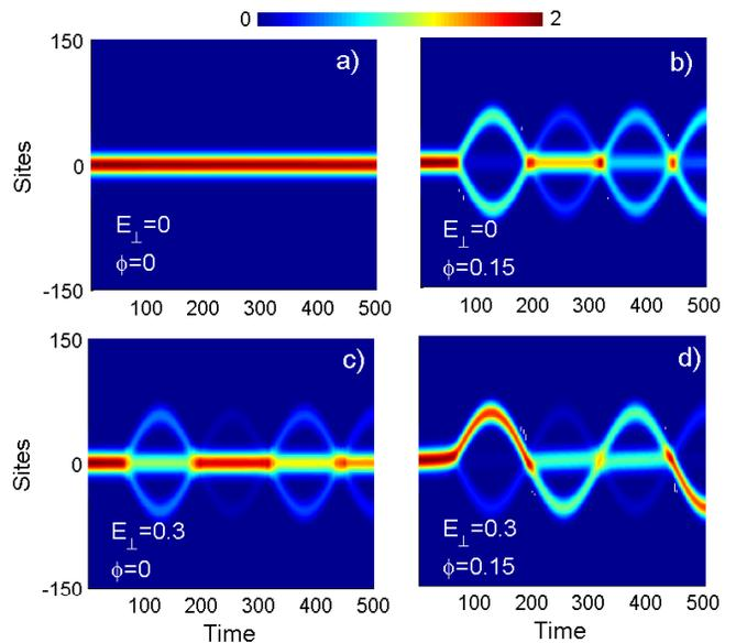
FIG. 5: Results of numerical simulations exciting initially the CLS in Fig.3(a), with respective field values as taken in graphs of Fig. 4. In all simulations  $E_{\parallel} = 0.05$ . The space-time evolution of the norm density  $\rho_n = |a_n|^2 + |b_n|^2 + |c_n|^2$  is plotted in color code.
