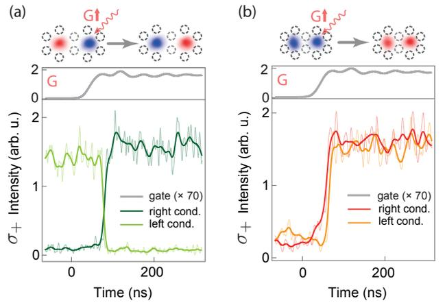
FIG. 4. (a) Spin switching for AF-coupled condensates. The  $\sigma_+$ -polarized gate is applied on the right condensate (shown above). The condensate-pair switches from  $|\uparrow\downarrow\rangle$  to  $|\downarrow\downarrow\rangle$ . (b) Spin switching for F-coupled condensates. The condensate-pair switches from  $|\downarrow\downarrow\rangle$  to  $|\uparrow\uparrow\rangle$ . The top panels show the gate laser intensity profile G. The gate laser is turned on at  $t = 0$ .
