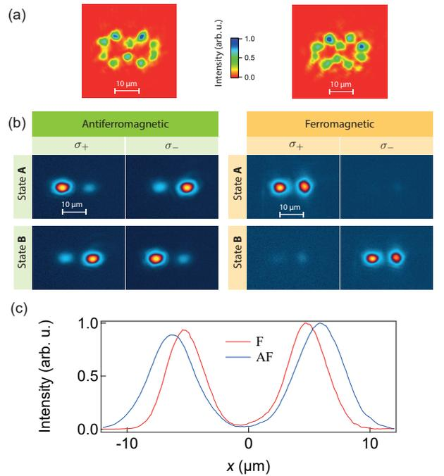
FIG. S1. (a) Pump intensity profiles in AF(left) and F-regimes (right) (b) Polarization-resolved real-space PL in AF (left) and F regimes (right). (c) Intensity profiles of the total emission in F and AF regimes.
