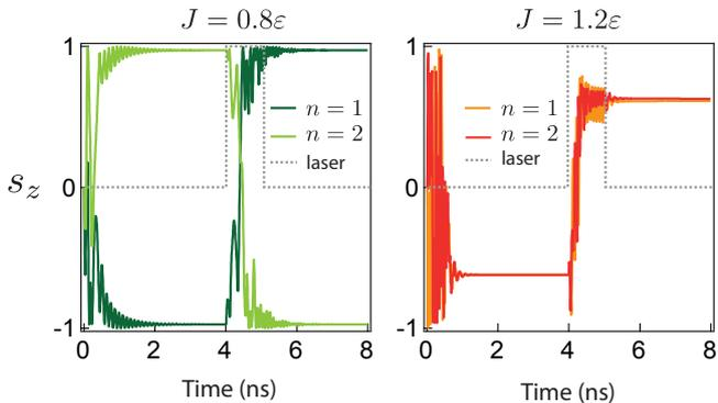
FIG. S6. The time evolution of two condensates for the case when  $J = 0.8\varepsilon$  (a) and  $J = 1.2\varepsilon$  (b) is shown. The condensate-pairs switch their spin states when a gate pulse with an opposite spin is applied on condensate 1. The gate pulse is a spin-up square pulse that is turned on at  $t = 4$  ns and lasts for 1 ns. Parameters as in text with  $|F|/\sqrt{N} = 7.5 \times 10^{-3}$ , where  $N$  is the occupation of the condensates with  $\omega_g$  at the condensate energy.
