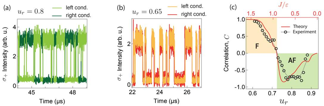
FIG. 3. (a,b) Snapshot in time of left and right condensate  $\sigma_+$  intensities for (a)  $u_r=0.80$  and (b)  $u_r=0.65$ , showing spontaneous correlated flipping of both condensates spins in (a) AF and (b) F regimes. (c) Magnetic phase diagram, with measured correlation  $C$  between magnetization of condensates 1,2 as a function of barrier  $u_r$  (circles, dotted line is guide for the eye). Simulations give the correlation  $C$  as a function of  $J/\varepsilon$  (red line).
