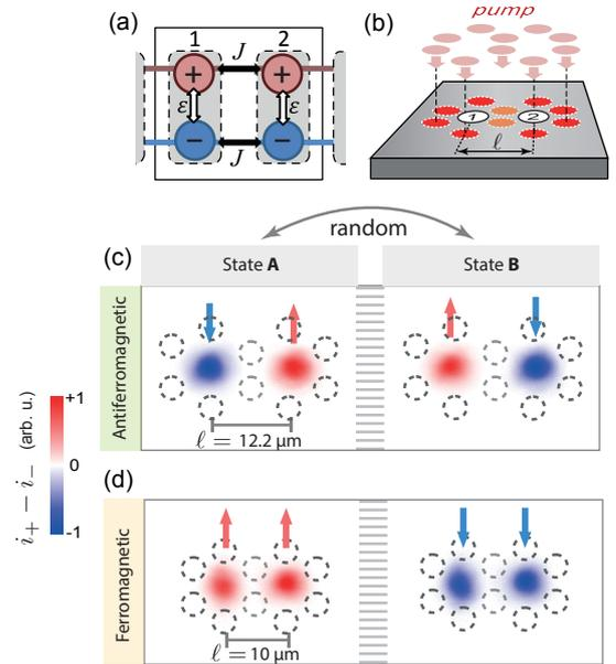
FIG. 1. (a) Coupling between condensates 1,2 controlled by Josephson tunneling  $J$ , spin-coupling ( $+$   $\leftrightarrow$   $-$ ) within condensates controlled by energy splitting  $\varepsilon$ . (b) Schematic double condensate trap from 10 pump beams. (c,d) Experimental spin states seen for (c) AF- and (d) F-coupled condensates. In each case two possible states exist, with actual state chosen randomly upon each realization.
