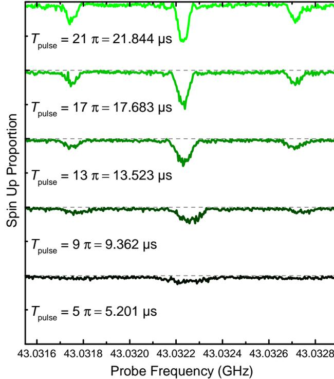
Figure S1: **Dressing the electron spin.** Mollow spectra of the dressed electron spin for different microwave pulse lengths. Here, a strong, resonant driving field  $P_{\text{pump}}$  was used to dress the spin state, while a weaker probe field  $P_{\text{probe}} = P_{\text{pump}} - 26$  dB was scanned over the Mollow triplet to record the spectra.
