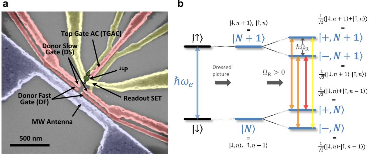
Figure 1: **Sample design and energy level diagram.** **a**, Scanning electron microscope image of a device, similar to the one used for measurements. Highlighted are the positions of the  $^{31}\text{P}$  donor, the donor gates, the microwave (MW) antenna, and the single electron transistor (SET) for spin readout. **b**, Energy level diagram of the electron spin subsystem in the spin picture and the dressed picture.
