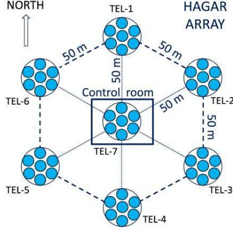
**Fig. 1.** Schematic of the HAGAR telescope array. The hexagonal array has a radius of 50m, and each telescope has 7 PMTs in a hexagonal array.
