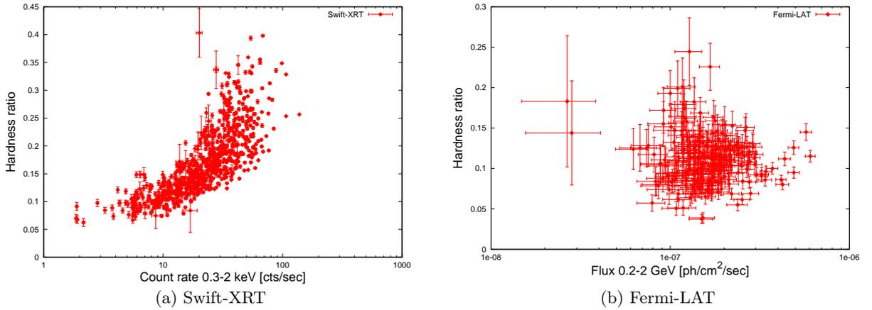
**Fig. 4.** Hardness ratio in the X-ray(Swift-XRT) band and GeV (Fermi-LAT) bands. While the trend of spectral hardening with flux is clear in the X-ray band, no such trend is seen in the GeV band.
