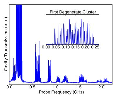
Fig. 5. Spectroscopy of the cavity in a near-degenerate configuration wherein the first even mode becomes degenerate with the fundamental. Inset: zoomed-in spectrum of the first clump of degenerate modes.
