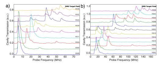
Fig. 6. Cavity transmission when the cavity is pumped by fields created by DMD masks of ideal HG-modes. a) Even mode spectra. b) Odd mode spectra.
