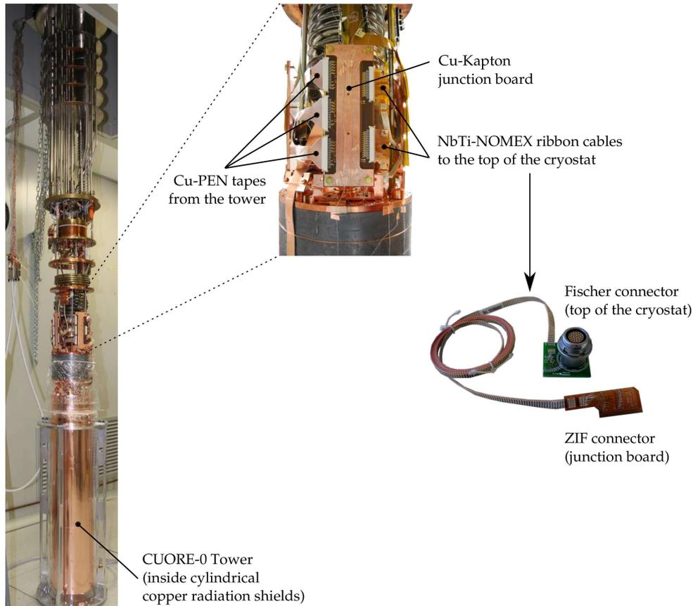
**Figure 14.** Photograph of the CUORE-0 tower attached to the dilution refrigerator, before the installation of the thermal radiation shields. Right: A zoom of a Cu-Kapton junction board, which connects the Cu-PEN cable to the NbTi-NOMEX cables which run up to the top of the cryostat.
