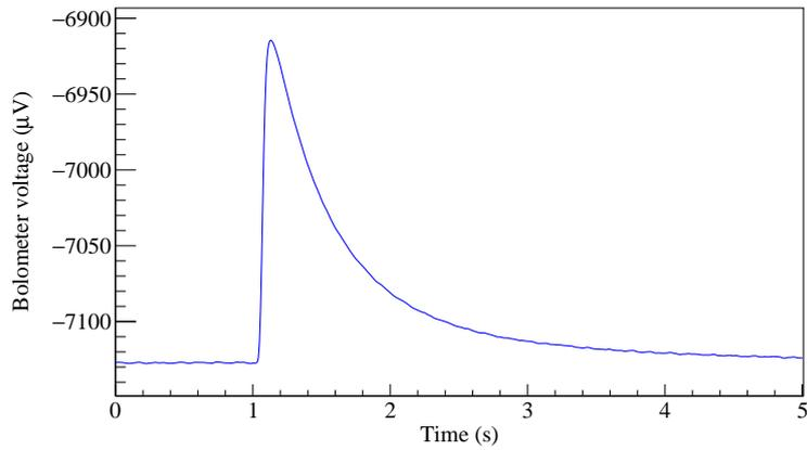
**Figure 22.** A pulse detected by a CUORE-0 bolometer, generated by an energy release of about 2615 keV during a calibration run. The voltage reported is referred to the ends of the NTD sensor, which was polarized with a current of  $\sim 250$  pA.
