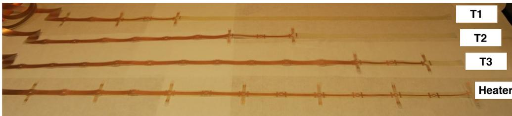
**Figure 7.** The four types of CUORE-0 Cu-PEN tapes. The picture shows the bottom ~80 cm of the tapes that were located on the sides of the tower.
