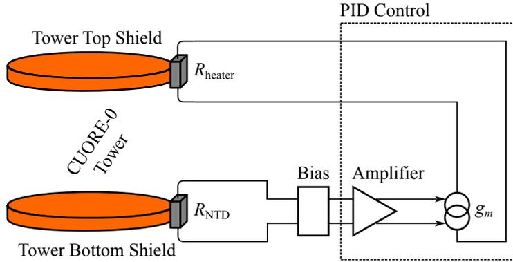
**Figure 17.** Temperature stabilization set-up of the CUORE-0 tower.
