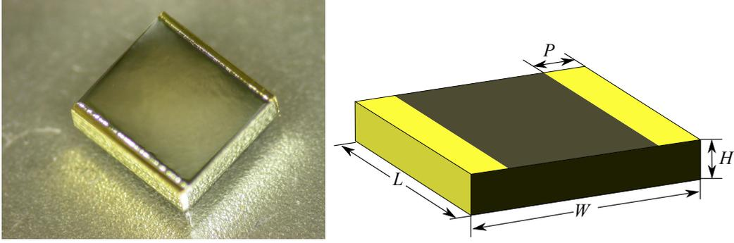
**Figure 4.** Left: Photograph of a CUORE-0 thermistor. Right: Diagram of the wrap-around thermistor geometry. Typical values for the dimensions are  $L = 3.0$  mm,  $W = 2.9$  mm,  $H = 0.9$  mm and  $P = 0.2$  mm.
