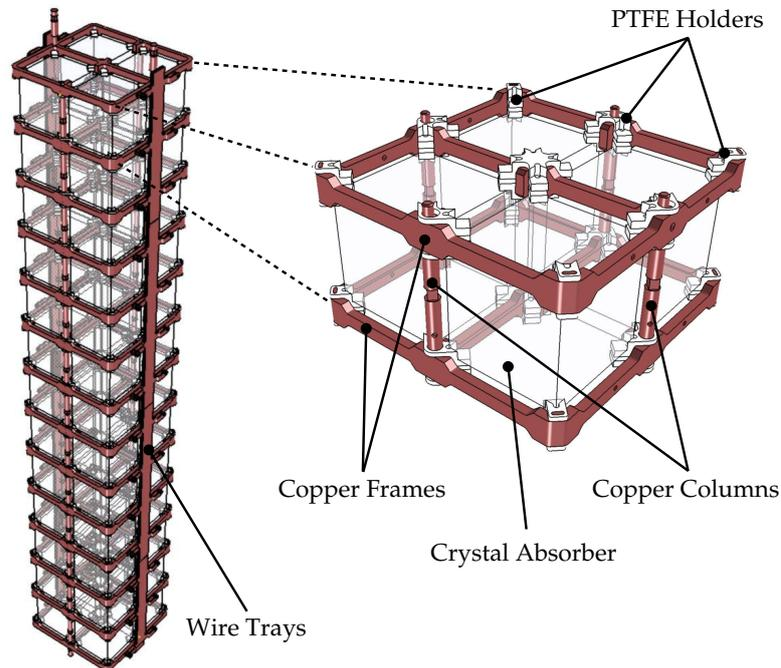
**Figure 2.** Left: A rendering of the CUORE-0 tower, including the wire trays for signal connection. Right: A single CUORE-0 detector floor, in which the  $\text{TeO}_2$  crystals, PTFE holders, and copper frames and columns are indicated. The copper frames are shared between adjacent floors.
