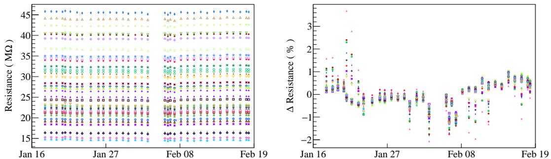
**Figure 23.** Left: Values of the CUORE-0 bolometer resistances at the working point measured daily over a period of one month in 2014. Right: Percentage variation of the same resistance values over the same time period. In both plots different marker colors and styles identify different bolometers.
