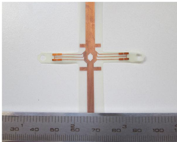
**Figure 8.** Detailed view of copper pads onto which the gold wires were bonded. The width of each copper track is 0.2 mm with a pitch of 0.4 mm. The total width of the tape is 13.4 mm, with a 1.0-mm minimum margin on each side.
