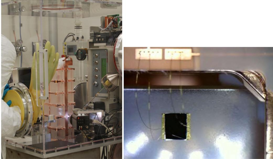
**Figure 12.** Left: The assembly workstation during the bonding operations. The bonding machine is on the right of the picture. Right: Detail of the bonding connection of a NTD thermometer. The gold pads of the thermistor are connected to the copper pads of the Cu-PEN cable through gold wires.
