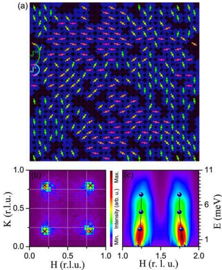
**Figure 6.** (a) Spin structure calculated for  $x \sim 0.7$ . The black spheres represent  $\text{Co}^{3+}$  LS ions, and the colored spheres with the arrows indicate  $\text{Co}^{2+}$  HS ions with spins. (b) Corresponding magnetic neutron scattering intensities in the  $HK0$  plane: crosses signify experimental peak positions for  $x = 0.7$ . (c) Magnetic excitation spectrum together with the experimentally observed values for this Sr doping (circles).
