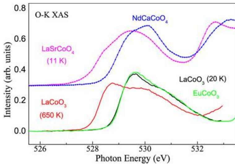
**Figure 3.** O-K X-ray absorption spectra of LaSrCoO<sub>4</sub> at 11 K (magenta), NdCaCoO<sub>4</sub> at 300 K (blue), LaCoO<sub>3</sub> at 650 K, and 20 K (red and black) and EuCoO<sub>3</sub> at 300 K (green).
