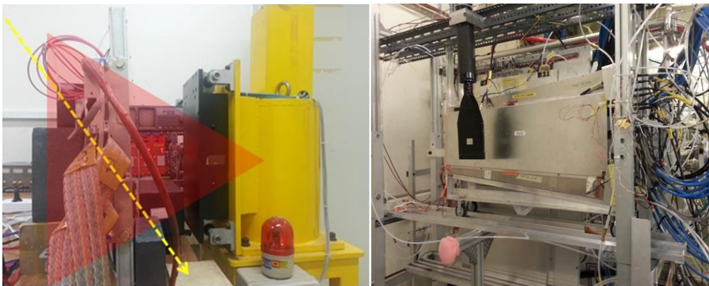
Fig. 3. Prototype RPCs installed at a distance of 36 cm from the 5.55-GBq ^{137}\text{Cs} source at Korea University (left), and at about 5 m from the 13.9-TBq ^{137}\text{Cs} source at the GIF++ (right).
