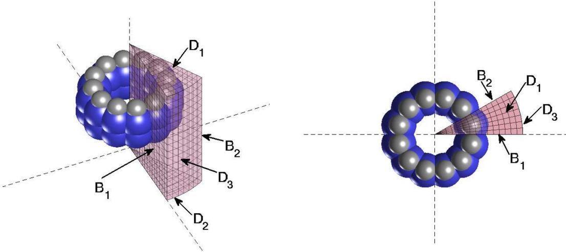
(b) The symmetry cell reduction results in cyclic-Bloch boundary conditions for the orbitals and cyclic boundary conditions for the density on the surfaces  $B_1, B_2$ . Both the electron density and the orbitals are subjected to zero-Dirichlet boundary conditions on the surfaces  $D_1, D_2, D_3$ .
