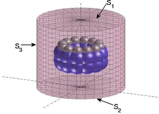
(a) The original problem for the cyclic structure posed in the cylinder  $\mathcal{C}$ . The orbitals and the electron density are subjected to zero-Dirichlet boundary conditions on the surfaces  $S_1, S_2, S_3$ . On these surfaces, the electrostatic potential is given by Eq. 8c. Note that  $\partial\mathcal{C} = S_1 \cup S_2 \cup S_3$  in the notation of the text.
