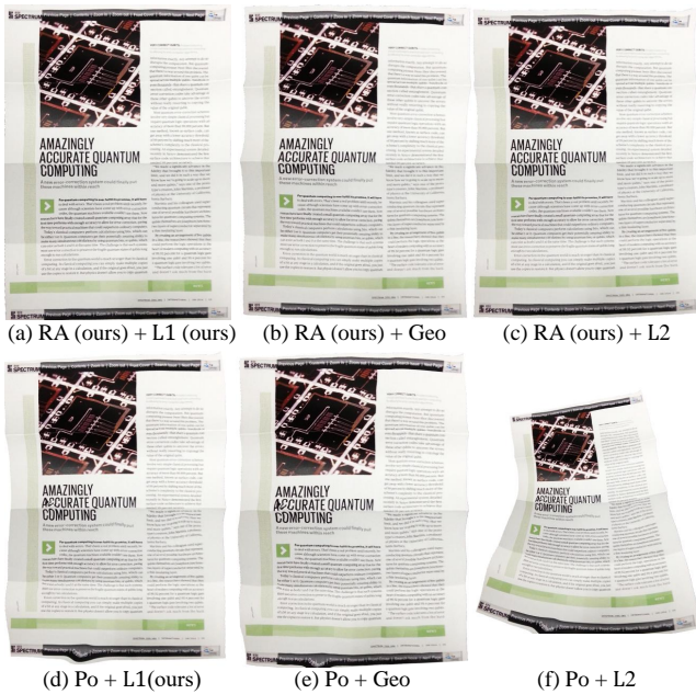
Fig. 5. Rectification results from combination of methods. Acronyms RA and Po denote our ridge-aware method and Poisson reconstruction respectively. L1 denotes our \ell_1 conformal mapping method with non-local constraints; L2 indicates LSCM [29] and Geo indicates geodesic unwrapping [30]. Po + L2 produced gross failures and is thus not compared.
