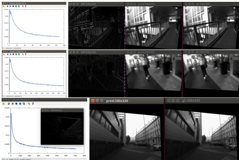
**Fig. 3.** Training results on pure rotation motion. The graphs show how the training error decreases as number of epochs increase. This serves as a sanity check for our network that includes many new layers that we propose in this library. The improvement in the training is qualitatively evident from the difference images: early stages in the optimisation show high residual in the registration but as more epochs are thrown to the optimisation, the residual error gracefully decreases.
