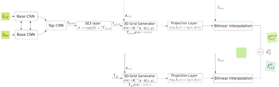
**Fig. 2.** We train a siamese network to regress to the relative pose vector between the two consecutive frames,  $I_{ref}$  and  $I_{live}$ . This pose vector is turned into a  $3 \times 4$  transformation matrix that transforms 3D points coming from the 3D grid generator and further projected into a 2D plane via projection layer which are used to generate a warped image. Additionally, the 3D grid generator needs an explicit depth-map as input to generate 3D points for any 3D warping.
