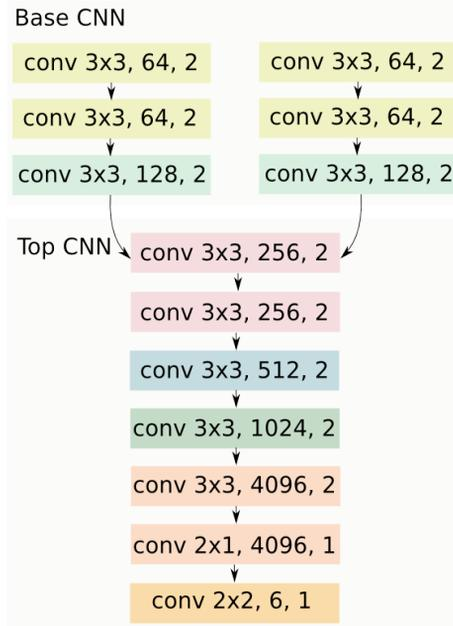
**Fig. 1.** Our Siamese network is inspired by the popular VGG-16 network [16] where  $3 \times 3$  convolutions are used in most layers and works for  $320 \times 240$  image resolution. Each convolution layer is followed by PReLU non-linearity [17]. We explicitly avoid any pooling and use a stride of 2 in every convolution layer for any downsampling.
