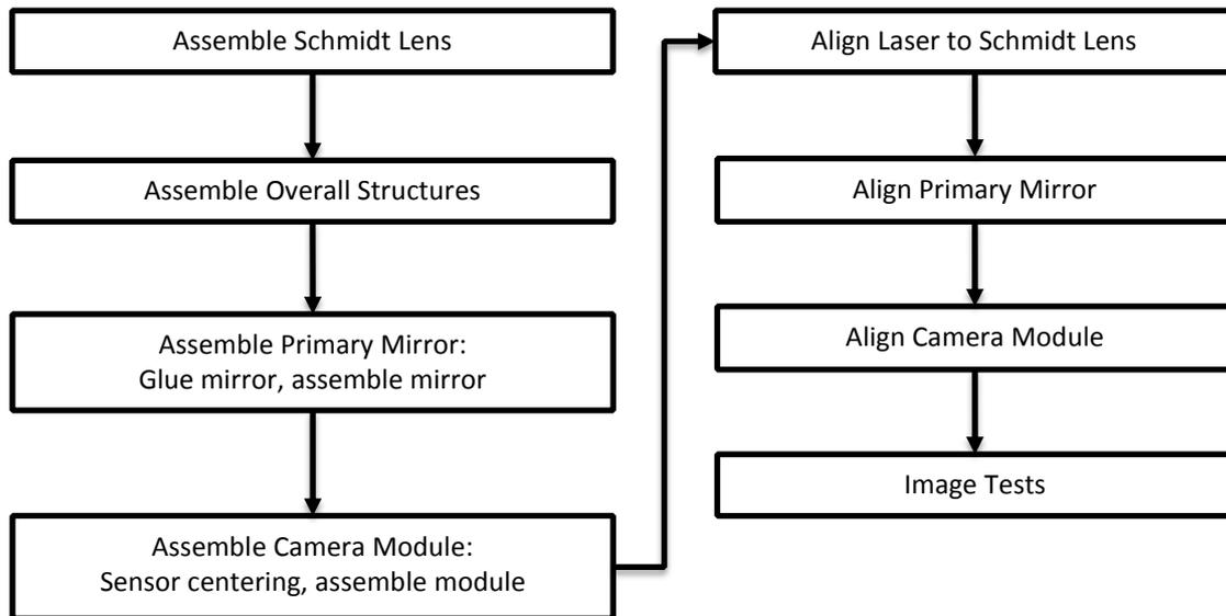
Figure 11. Flow chart of the metrology camera integration and testing procedure in the laboratory.
