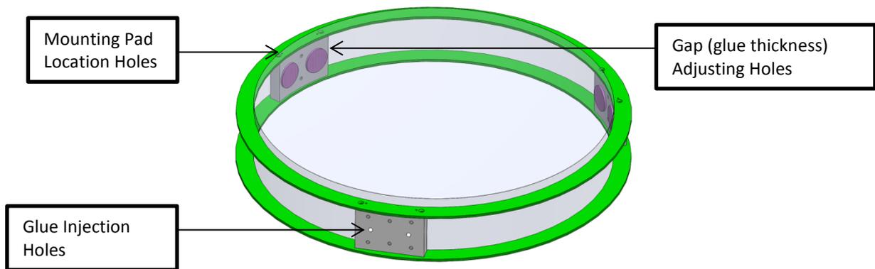
Figure 13. Device used for mirror mounting pads installation.
