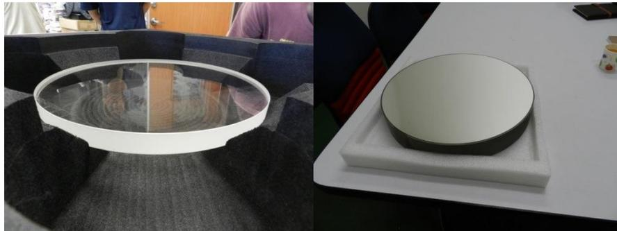
Figure 3. The left panel shows the Schmidt plate fabricated by Nikon Corporation. The right panel shows the spherical mirror fabricated by Control Optics Taiwan Inc.
