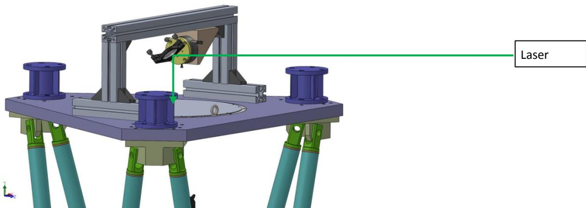
Figure 14. A fold mirror will be set on top of the Schmidt lens holder for the alignment process.
