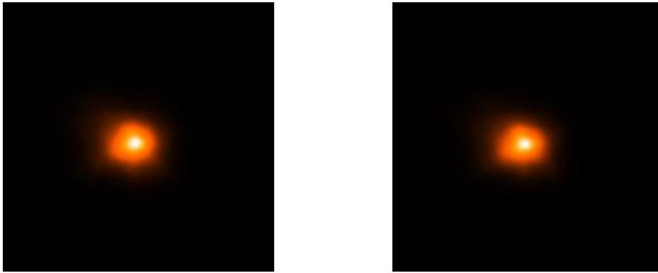
Figure 2. As-built PSF for field center (left) and field edge (right) of the PFS metrology camera after considering all degradation factors.
