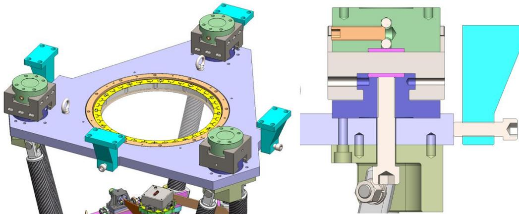
Figure 10. Left panel shows the top view of the three connection mechanisms between the Schmidt plate and the Cassegrain box. Right panel shows the cross section view of one adjusting mechanism. Two screws inside the adjusting mechanism are used to lock the movement of the mechanism; one screw inside the cyan block is used to adjust the centering of the metrology camera.
