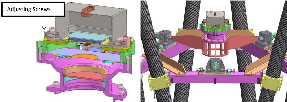
Figure 7. Left panel shows the side view of camera module. From top to bottom are the Canon 50M camera (grey), camera adapting board (green-yellow), shutter cell (green) and lens cell (pink). Right panel shows an overall view of the camera module supporting structure.
