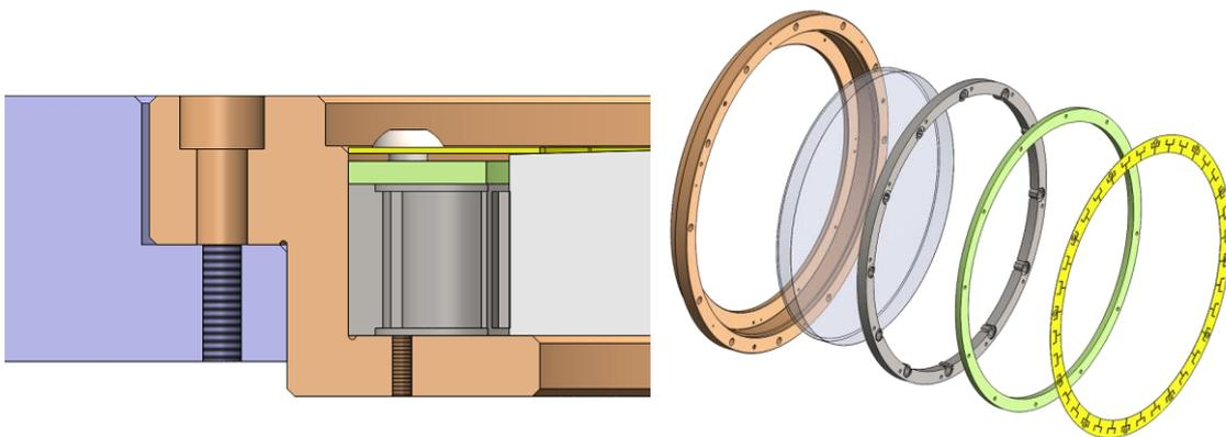
Figure 5 left: Side view of the Schmidt plate holder. From top to bottom are the steel disc spring (yellow), aluminum spacer ring (green), steel roll-pin flexure and steel Schmidt plate holder (brown). Right: The explosive view of the Schmidt plate holder.
