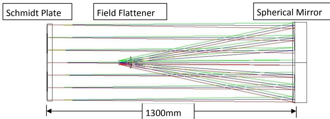
Figure 1. The optical layout of the metrology camera.
