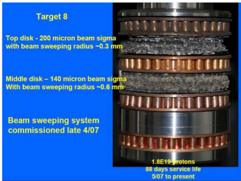
FNAL's pbar production target
