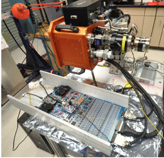
Figure 18. GLS Scientific cryostat (orange) with the SAPHIRA detector installed inside and the PB1 (“PizzaBox”) electronics circuit board (blue) in the lab in Hilo, Hawai’i.
