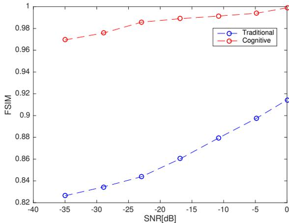
Fig. 16: Comparing between traditional and cognitive SAR images using the FSIM index.
