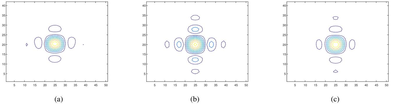
Fig. 5: A point spread function (PSF) of a SAR system simulated with different RDA techniques (range is the vertical axis and azimuth is the horizontal one). (a) Conventional RDA, PSLR = 13.32 [dB]. (b) Fourier domain RDA,  $|\nu(k, l)| = 3$ , PSLR = 11.7598 [dB]. (c) Fourier domain RDA,  $|\nu(k, l)| = 5$ , PSLR = 13.29 [dB].
