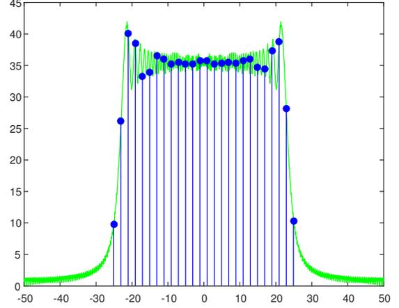
Fig. 4: Fourier series coefficients are taken within the effective bandwidth of the returned signals. Since the signals are finite in time the coherent information within the discrete frequency samples is sufficient to handle SAR processing.
