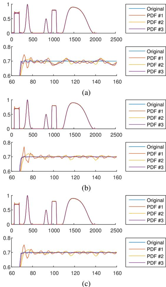
Fig. 9: One-dimensional signal reconstruction based on different subsampling strategies (paired with zoomed part). (a) Direct reconstruction using matched filtering. (b) Reconstruction with FISTA under the wavelet transform. (c) Reconstruction with FISTA under an identity transform.
