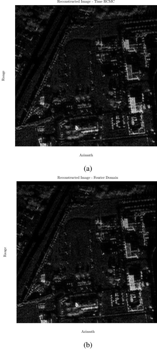
Fig. 7: Comparison between two reconstructed images. (a) Conventional RDA using oversampled raw data. (b) Fourier RDA,  $|\nu(k, l)| = 5$ , with no oversampling.
