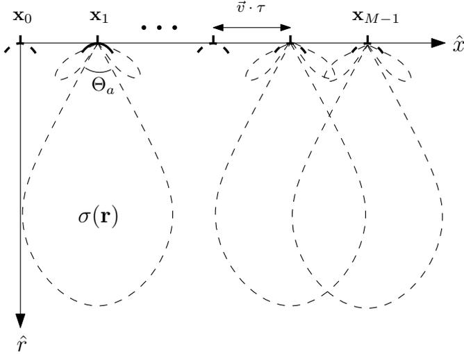
Fig. 1: SAR system model for the stripmap mode. The coherent information is recorded at different positions, spaced by a displacement of  $\vec{v}\tau$ . At every position the radar, which has an angular aperture of  $\Theta_a$ , captures a part of the scene reflectivity,  $\sigma(\mathbf{r})$ .
