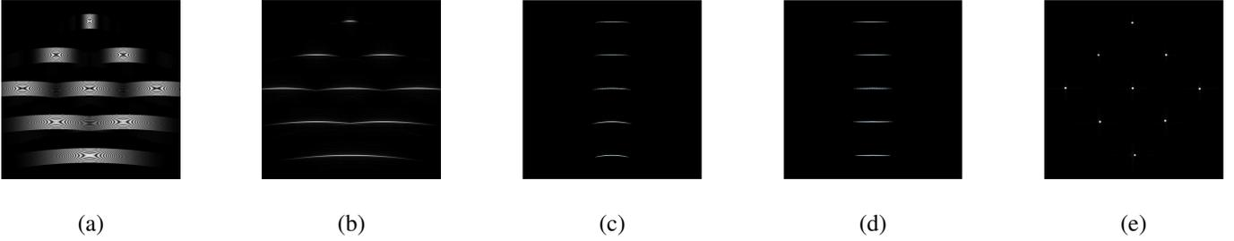
Fig. 2: The Range-Doppler Algorithm (RDA) stages for equally spaced single-point reflectors. (a) Raw data (real component). (b) Range compression. (c) Azimuth DFT. (d) Range cell migration correction (RCMC). (e) Compressed image.
