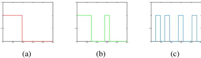
Fig. 8: Frequency bands selection. (a) Low pass (“PDF #1”). (b) A combination of low pass and a band pass (“PDF #2”). (c) Random selection (“PDF #3”).
